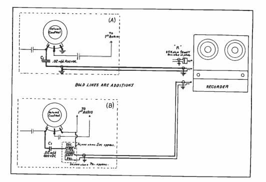
Figure 2. A—A simple connection that will work on most radio sets. The volume control is the best takeoff point for recording. Note 25,-000 ohm resistor which may be incorporated in the plug. B—For AC/DC sets and TV sets which may have a voltage on the chassis, it is necessary to hook up a transformer to prevent this voltage from reaching the recorder and causing hum. In stubborn cases, where ordinarily the hookup shown in A should be sufficient, B must be used instead.
