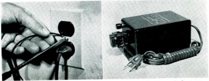
The Cornell-Dubilier AC line filter is shown at right. Into this is plugged a three-way adapter and all units, radio, TV and recorder plugged into it for best results. The terminal at the top of the case
