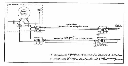
Figure 4. A—For long runs (up to 250 feet) transformers must be used at the source and at the recorder also. These are placed "back to back" with the low impedance sides connected to the line and the high impedance sides to the recorder and source. At B, the requirements for still longer lines (up to 500 feet) are shown.
