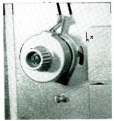
Constant tape tension is maintained by the arms. Automatic shutoff occurs at the end of a reel or if the tape should break.
