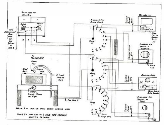
The drawing shows the hookup for the multiplegang switch. Note the connections for recording that have been made in the voice coil leads in the radio and TV set. The connections may be made to the volume controls of these units as is suggested and shown in the article that begins on the following page. All speakers used for playback should be of the permanent magnet type.
