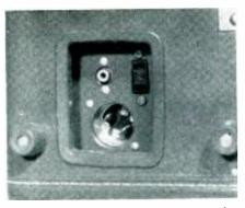
In this well in the side of the case can be found the power and audio inputs as well as a 110 volt output receptacle.
