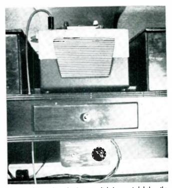
Close-up showing how the 3-gang switch is mounted below the recorder. The switches are available at radio parts supply houses and are not difficult to connect up.
