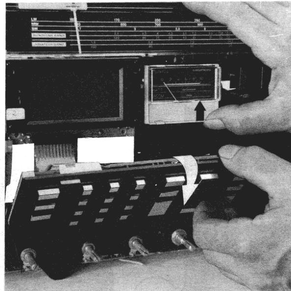
**Disassembly of Keyboard Panel and Digital Unit.**
