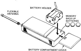
If you wish to use your PRO-30 with an external antenna such as a mobile antenna or outdoor base antenna, remove the flexible antenna and you can connect it to the BNC connector on the PRO-30.
