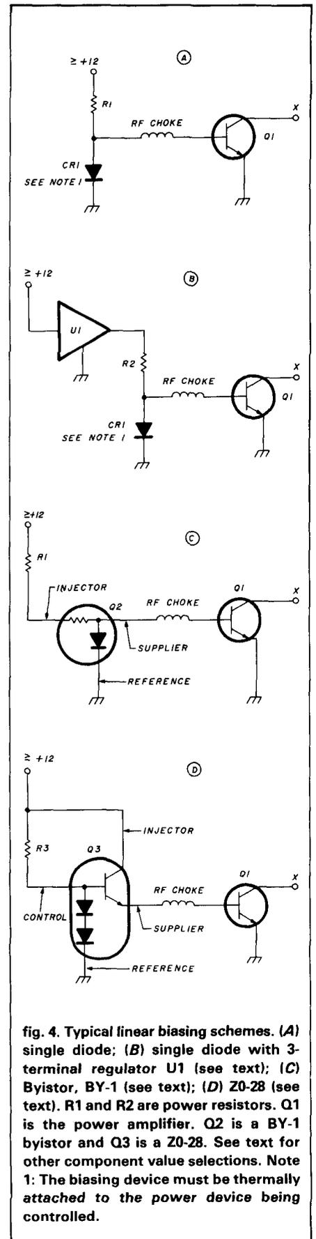
fig. 4. Typical linear biasing schemes. (A) single diode; (B) single diode with 3-terminal regulator U1 (see text); (C) Byistor, BY-1 (see text); (D) Z0-28 (see text). R1 and R2 are power resistors. Q1 is the power amplifier. Q2 is a BY-1 byistor and Q3 is a Z0-28. See text for other component value selections. Note 1: The biasing device must be thermally attached to the power device being controlled.
