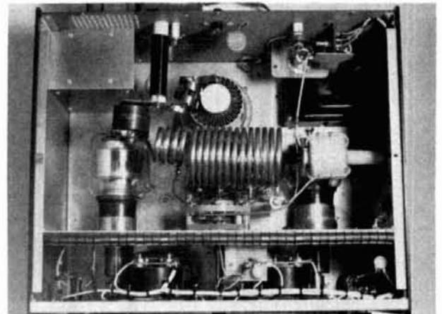
Top view of amplifier illustrates small size of 3CX1200A7. Compare it to the vacuum variables in the lower section of the photo.
