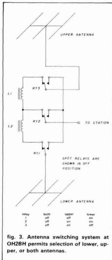
fig. 3. Antenna switching system at OH2BH permits selection of lower, upper, or both antennas.
