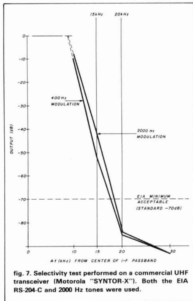
fig. 7. Selectivity test performed on a commercial UHF transceiver (Motorola "SYNTOR-X"). Both the EIA RS-204-C and 2000 Hz tones were used.
