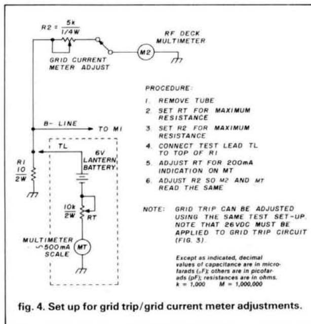
fig. 4. Set up for grid trip/grid current meter adjustments.
