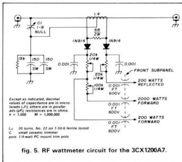
fig. 5. RF wattmeter circuit for the 3CX1200A7.
