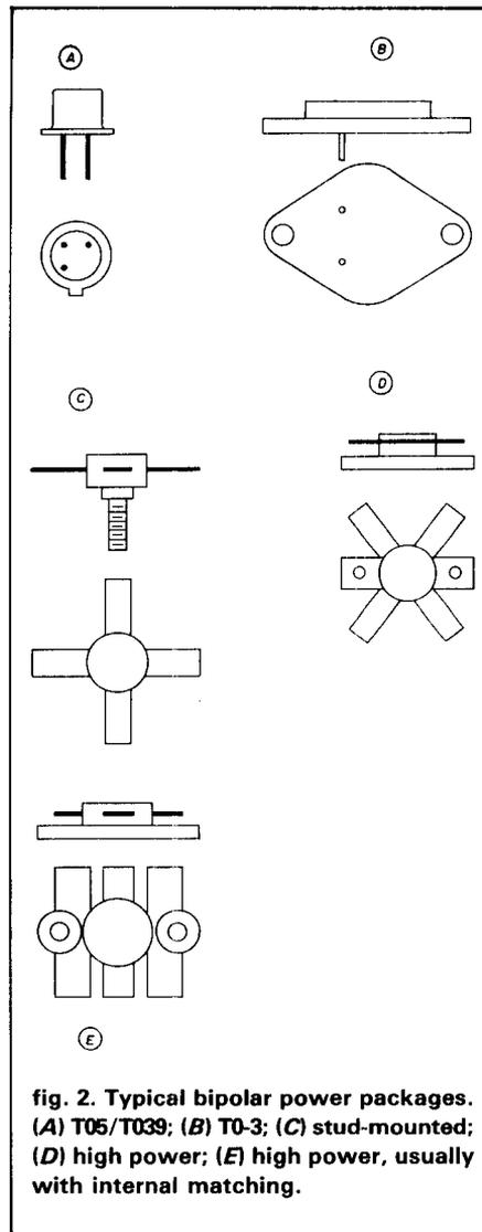
fig. 2. Typical bipolar power packages. (A) TO5/TO39; (B) TO-3; (C) stud-mounted; (D) high power; (E) high power, usually with internal matching.
