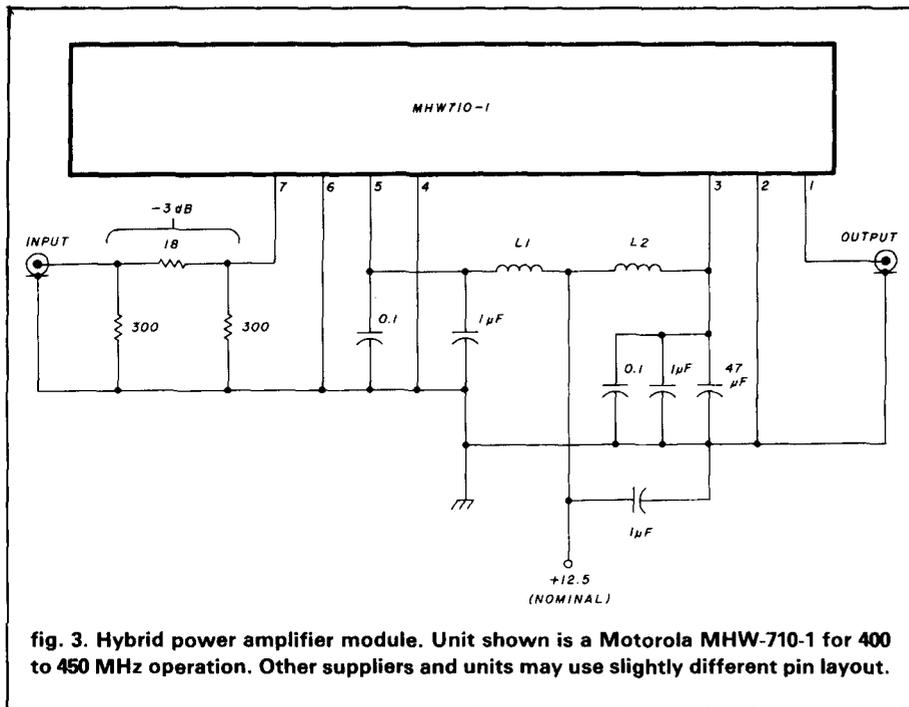
fig. 3. Hybrid power amplifier module. Unit shown is a Motorola MHW-710-1 for 400 to 450 MHz operation. Other suppliers and units may use slightly different pin layout.
