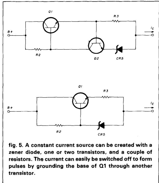
fig. 5. A constant current source can be created with a zener diode, one or two transistors, and a couple of resistors. The current can easily be switched off to form pulses by grounding the base of Q1 through another transistor.
