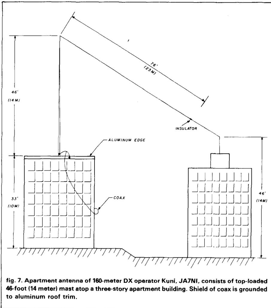
fig. 7. Apartment antenna of 160-meter DX operator Kuni, JA7NI, consists of top-loaded 46-foot (14 meter) mast atop a three-story apartment building. Shield of coax is grounded to aluminum roof trim.
