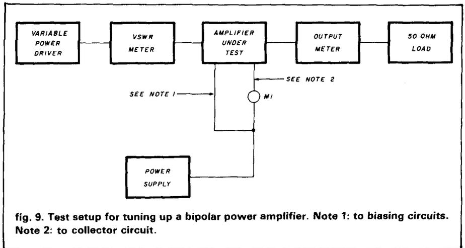
**fig. 9.** Test setup for tuning up a bipolar power amplifier. Note 1: to biasing circuits. Note 2: to collector circuit.
