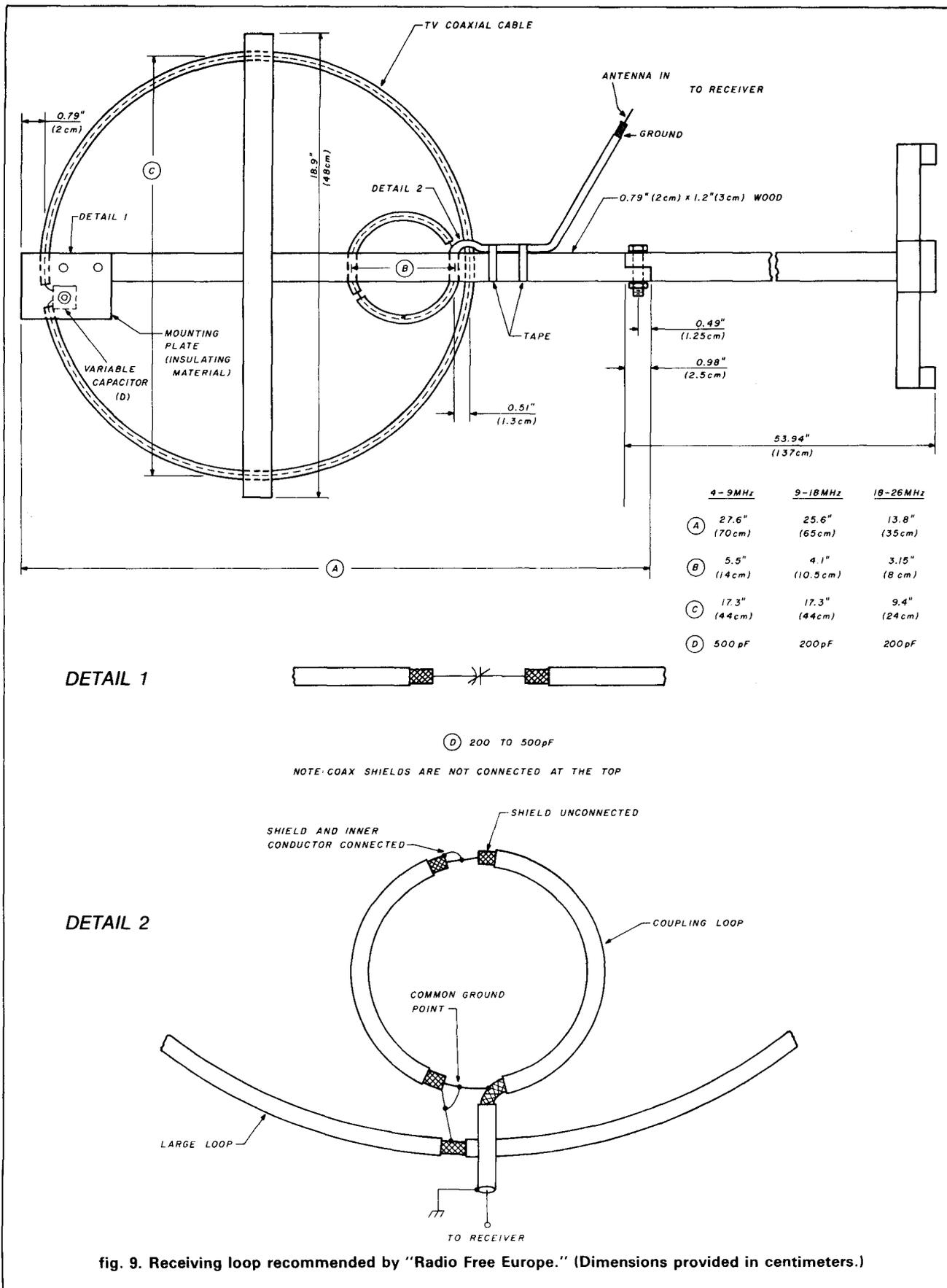
fig. 9. Receiving loop recommended by "Radio Free Europe." (Dimensions provided in centimeters.)
