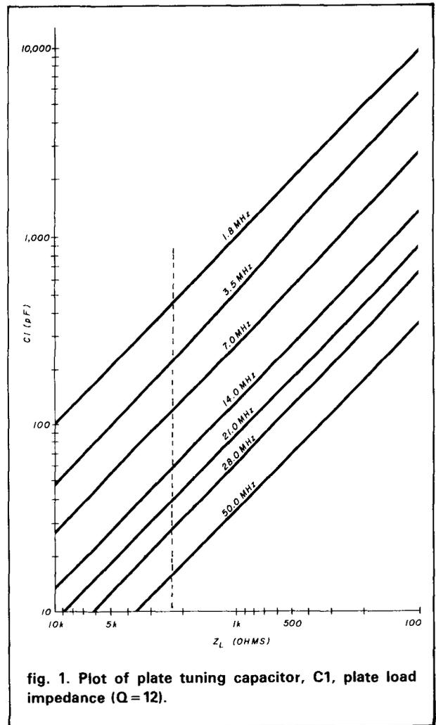
fig. 1. Plot of plate tuning capacitor,  $C_1$ , plate load impedance ( $Q = 12$ ).
