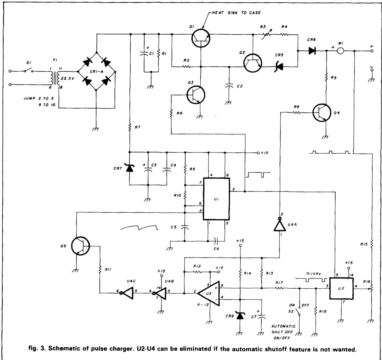
fig. 3. Schematic of pulse charger. U2-U4 can be eliminated if the automatic shutoff feature is not wanted.
