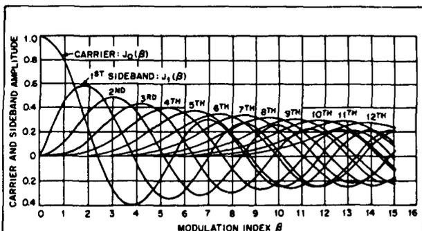
fig. 3. Plot of Bessel function of first kind as a function of argument  $\beta$ . (From P.F. Panter's *Modulation, Noise, and Spectral Analysis*, as reproduced in *Reference Data for Radio Engineers*, Sixth Edition, Howard W. Sams, Inc., publisher.)
