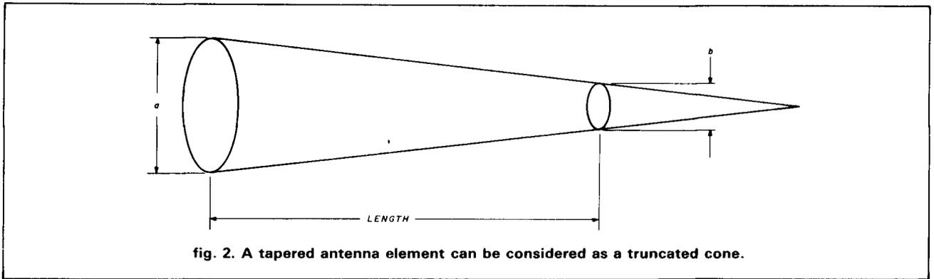
fig. 2. A tapered antenna element can be considered as a truncated cone.
