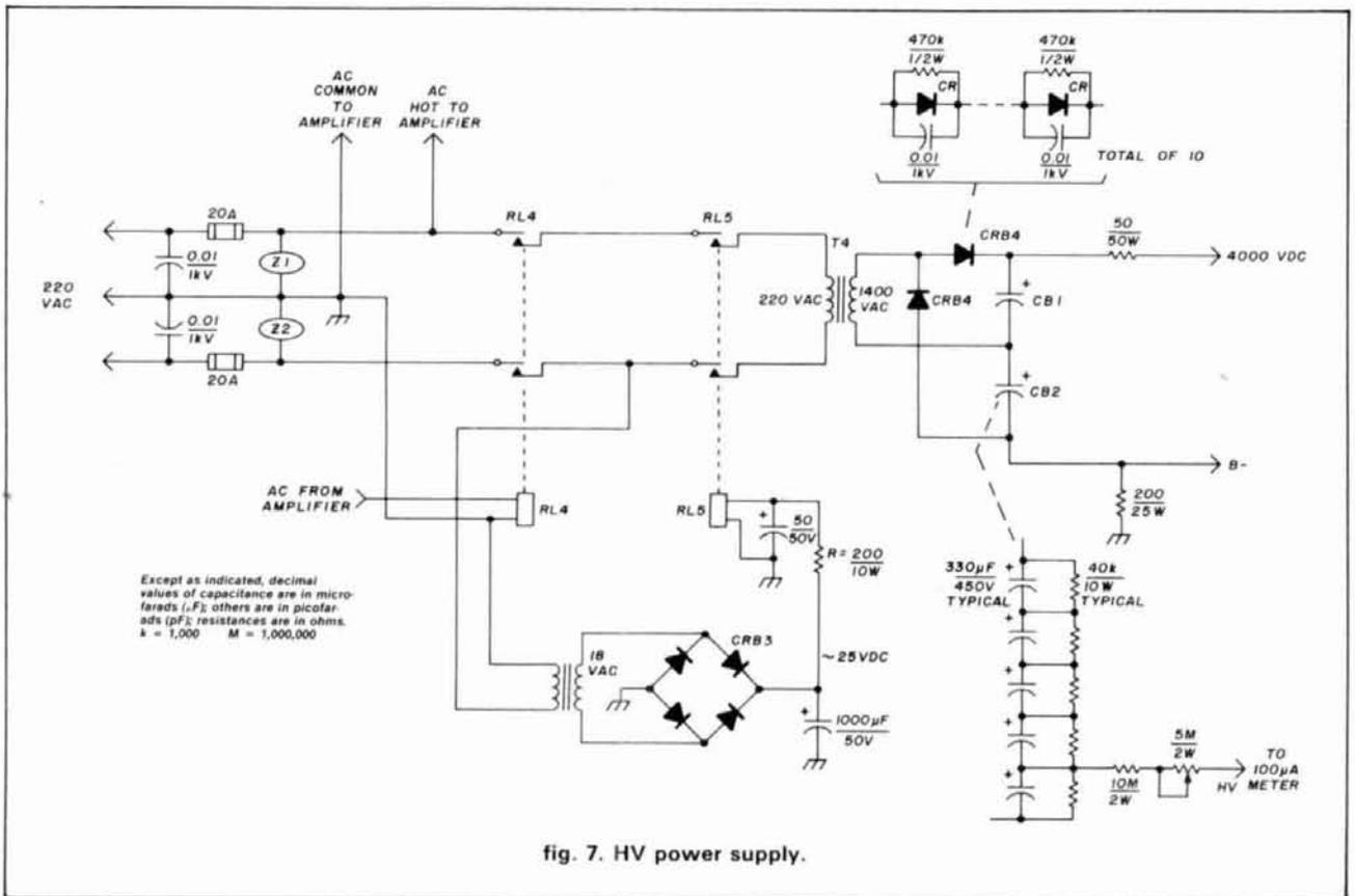
fig. 7. HV power supply.
