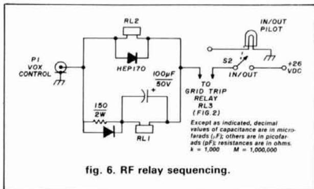
fig. 6. RF relay sequencing.
