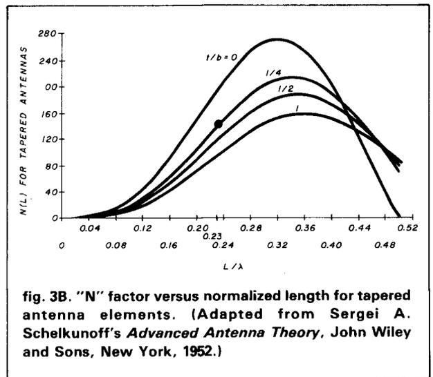
fig. 3B. "N" factor versus normalized length for tapered antenna elements. (Adapted from Sergei A. Schelkunoff's *Advanced Antenna Theory*, John Wiley and Sons, New York, 1952.)
