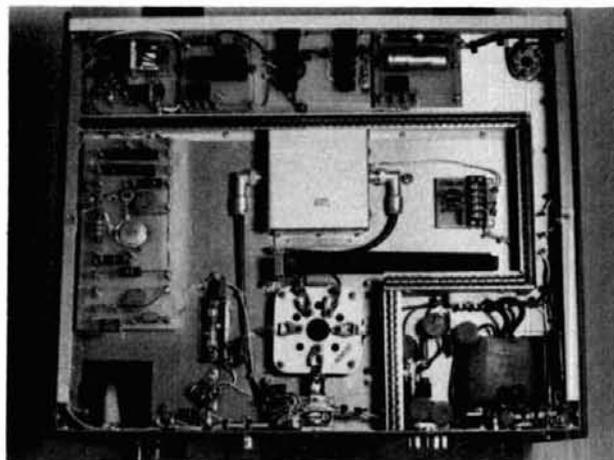
Bottom view of the amplifier illustrates the method used to isolate the RF circuitry from the control and power devices.
