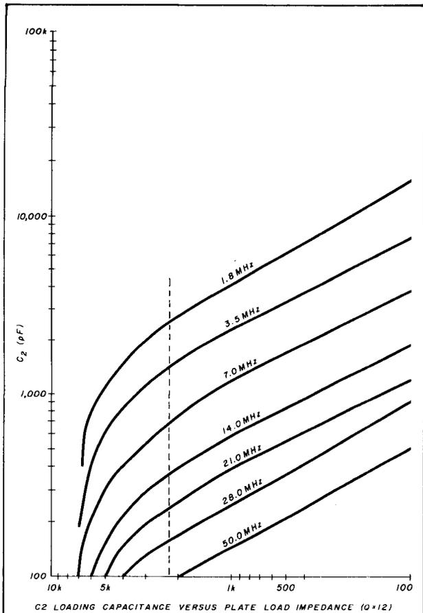
fig. 2. Loading capacitance versus plate load impedance (Q = 12).
