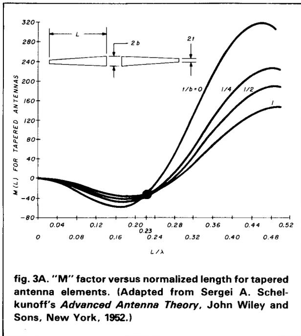
fig. 3A. "M" factor versus normalized length for tapered antenna elements. (Adapted from Sergei A. Schelkunoff's *Advanced Antenna Theory*, John Wiley and Sons, New York, 1952.)
