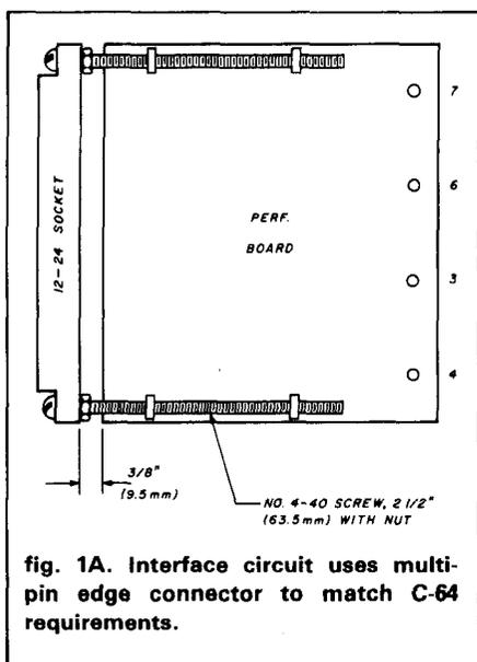
fig. 1A. Interface circuit uses multi-pin edge connector to match C-64 requirements.
