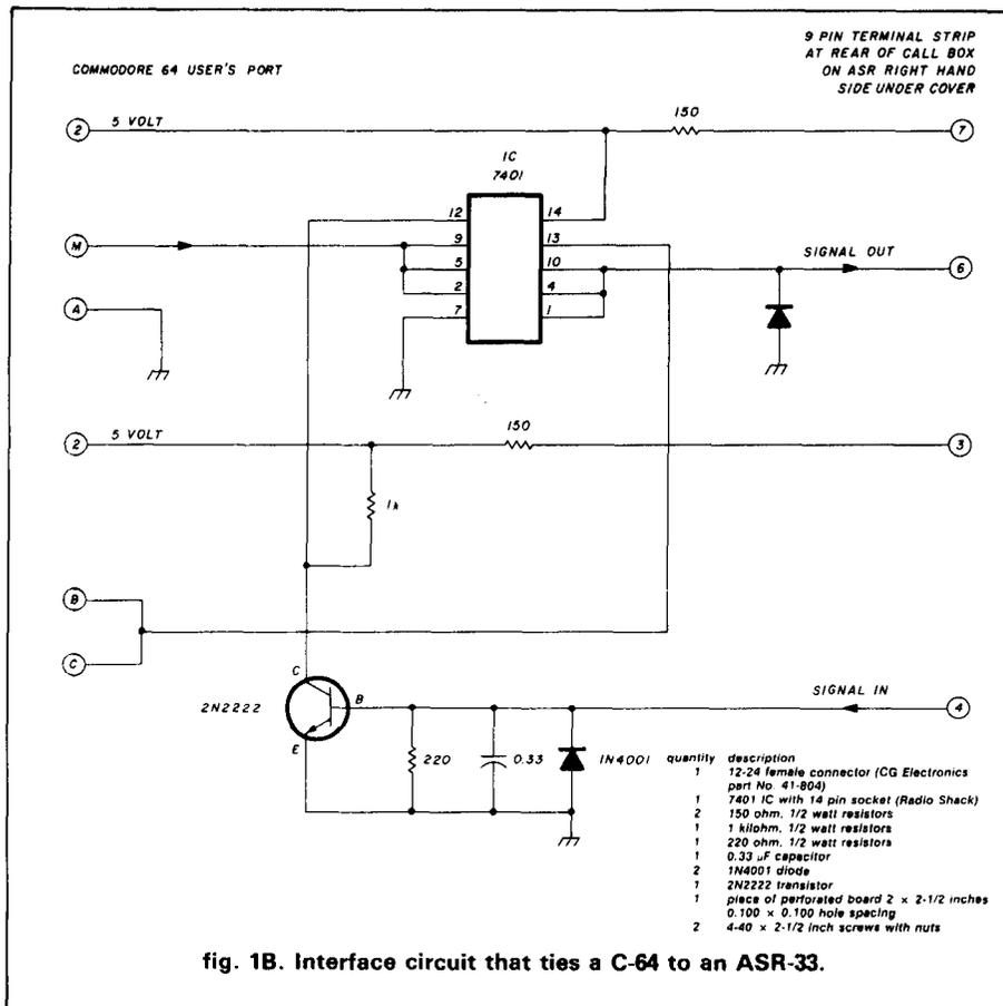
fig. 1B. Interface circuit that ties a C-64 to an ASR-33.
