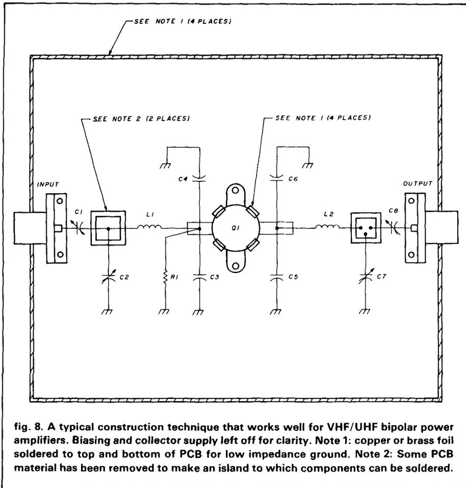
fig. 8. A typical construction technique that works well for VHF/UHF bipolar power amplifiers. Biasing and collector supply left off for clarity. Note 1: copper or brass foil soldered to top and bottom of PCB for low impedance ground. Note 2: Some PCB material has been removed to make an island to which components can be soldered.
