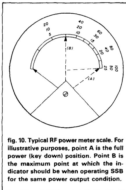
**fig. 10.** Typical RF power meter scale. For illustrative purposes, point A is the full power (key down) position. Point B is the maximum point at which the indicator should be when operating SSB for the same power output condition.
