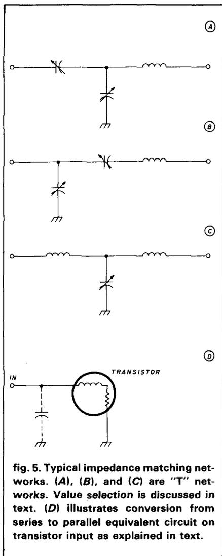
fig. 5. Typical impedance matching networks. (A), (B), and (C) are "T" networks. Value selection is discussed in text. (D) illustrates conversion from series to parallel equivalent circuit on transistor input as explained in text.
