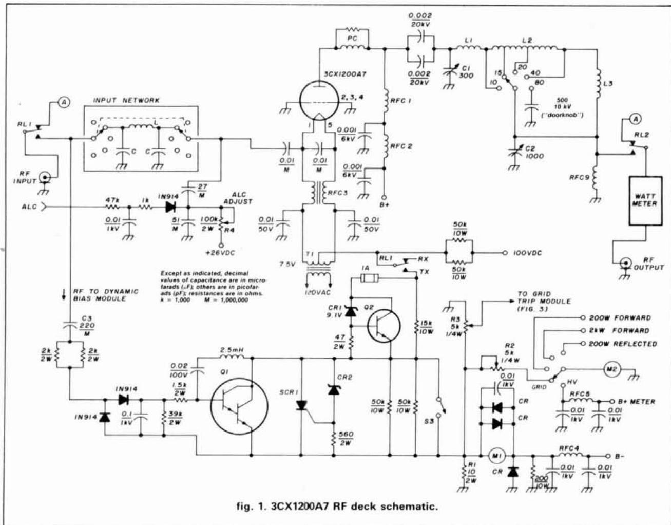
fig. 1. 3CX1200A7 RF deck schematic.
