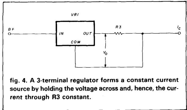
fig. 4. A 3-terminal regulator forms a constant current source by holding the voltage across and, hence, the current through R3 constant.
