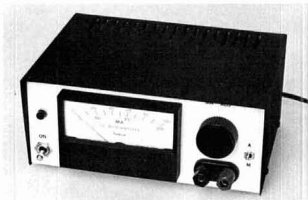
fig. 6. The charger fits nicely in a standard Radio Shack cabinet. Parts layout is not critical and any convenient construction method can be used.
