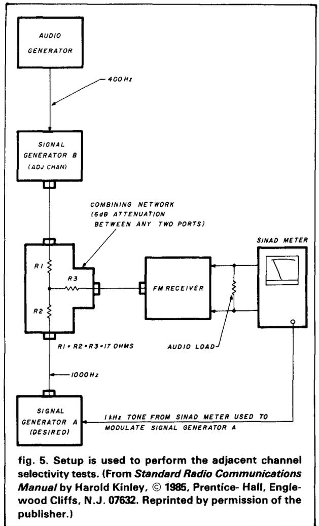
**fig. 5.** Setup is used to perform the adjacent channel selectivity tests. (From *Standard Radio Communications Manual* by Harold Kinley, © 1985, Prentice-Hall, Englewood Cliffs, N.J. 07632. Reprinted by permission of the publisher.)
