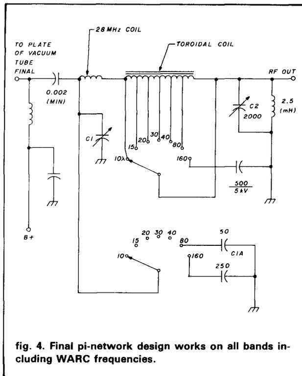
**fig. 4.** Final pi-network design works on all bands including WARC frequencies.
