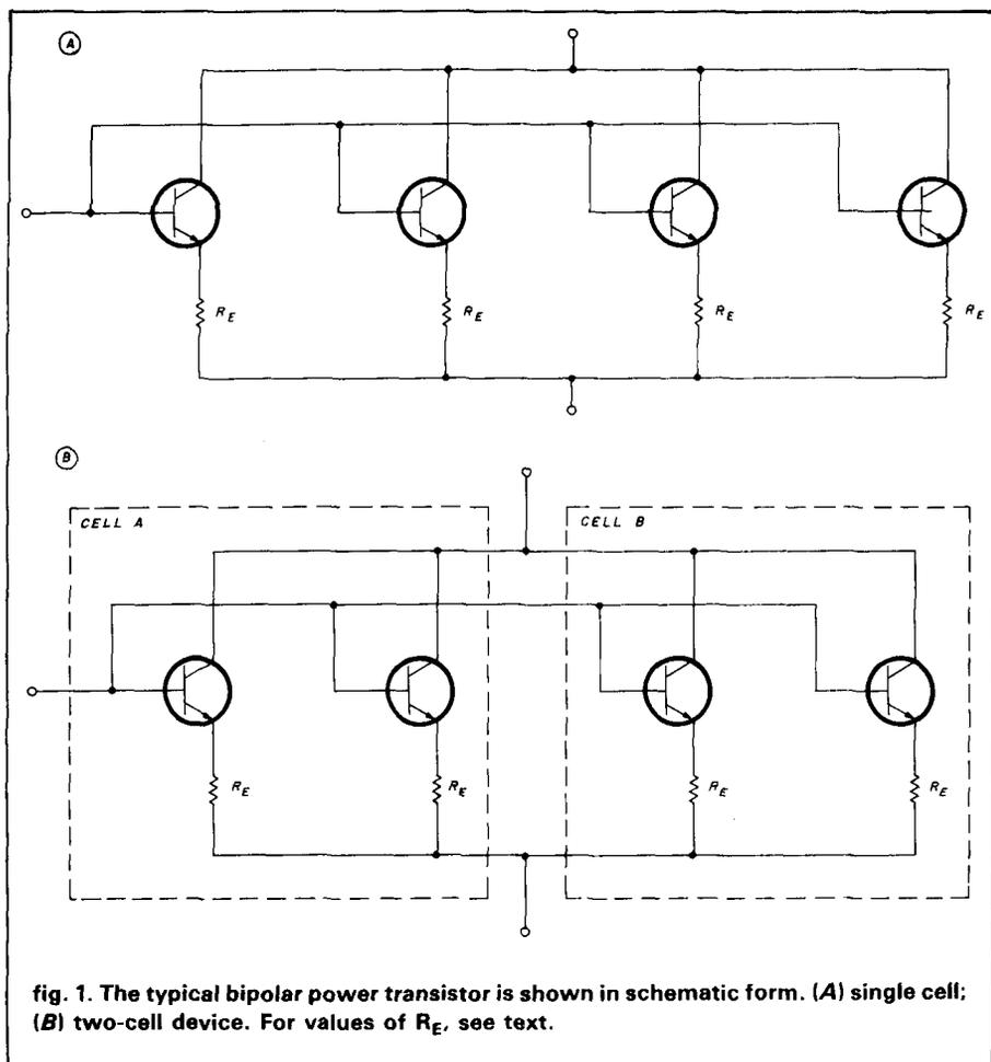
fig. 1. The typical bipolar power transistor is shown in schematic form. (A) single cell; (B) two-cell device. For values of  $R_E$ , see text.
