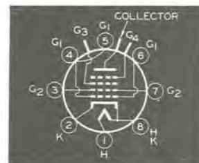
Bottom View of 825 Socket Connections
