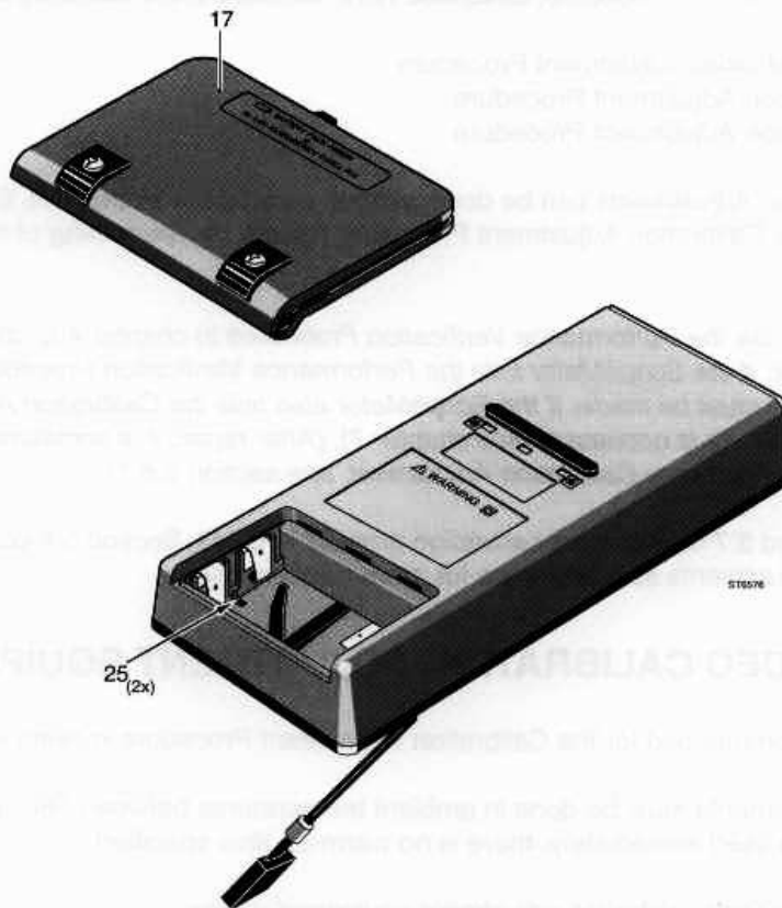
Figure 5.1 Position of the +12V and 0 contacts for calibration (items 25)
