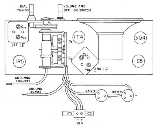
Output Meter - Connect Meter leads to the voice coil terminals of the speaker and turn the receiver volume control to maximum.
