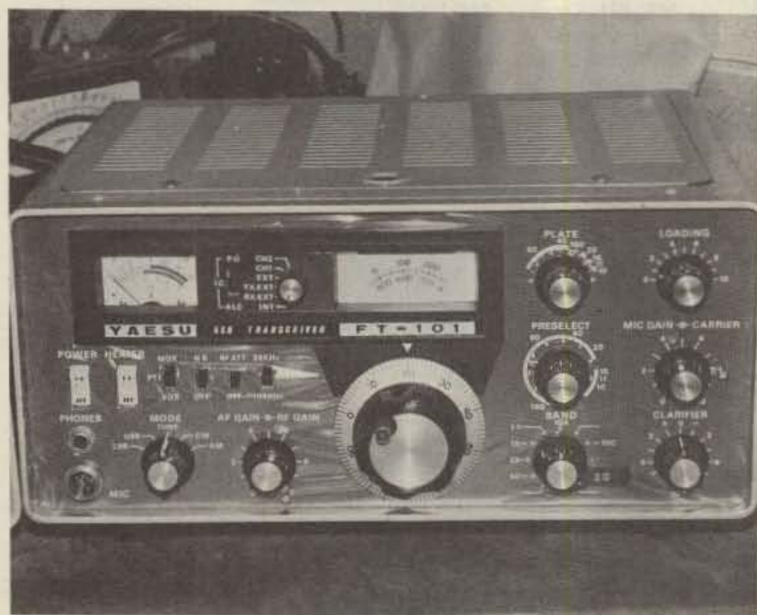
The outside appearance of the FT-101 remains essentially unchanged. Only the bottom cover plate and internal shield need be removed during the 30-meter modification. The position of all front-panel controls should be as shown after tuning up on 30 meters.
