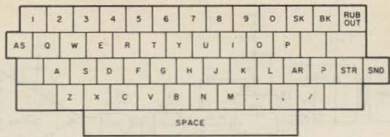
Fig. 1. The N7AGK ASR-33 Morse keyboard layout
