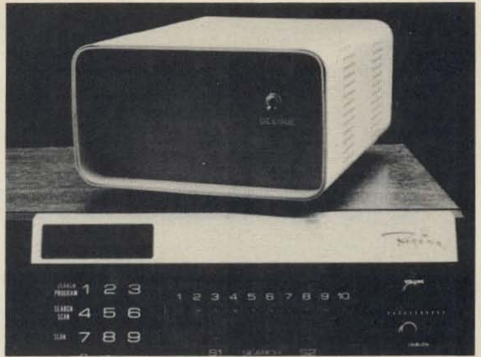
Overall view of the completed tone squelch. The squelch fits easily on top of the scanner.
