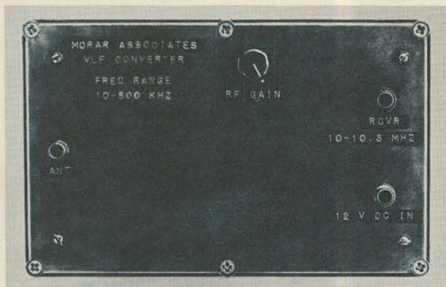
Photo A. Front panel, showing antenna input on left, 10 MHz out in the upper right, and 12 V dc input in the lower right. A tunable i-f output was added after this picture was taken (see the schematic). The tunable inductance core shaft was brought out as an operating control slightly to the right of the rf gain control. It can be seen in Photo C.
