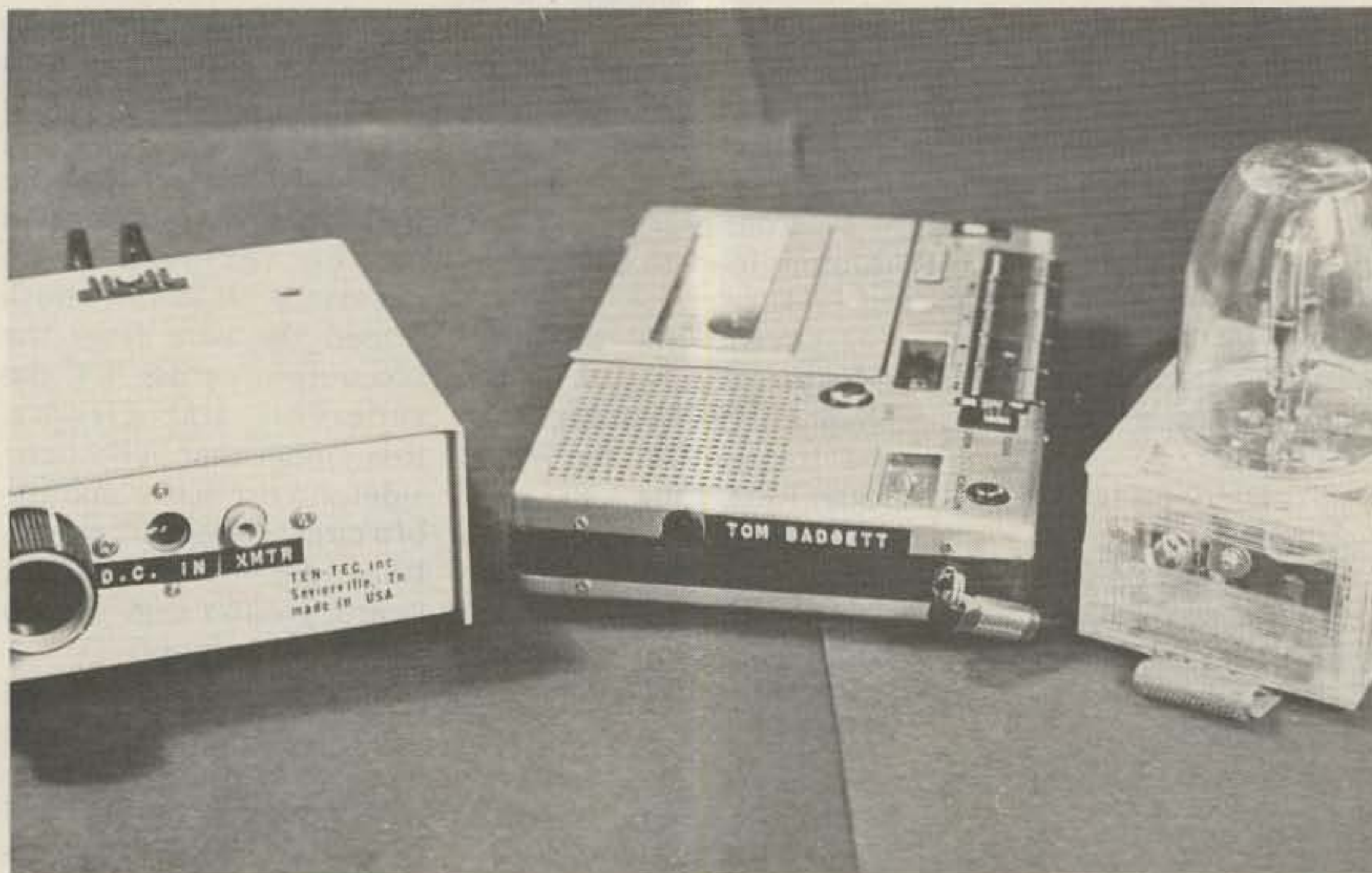
Here's some of the equipment I regularly power from a six-volt lantern battery. The keyer (left) is a Ten-Tec KR-1 paddle assembly with an Accu-keyer squeezed inside. My tape recorder is in the center, and on the right is a compact strobe I strap to my bicycle luggage carrier when I'm caught out after dark.
