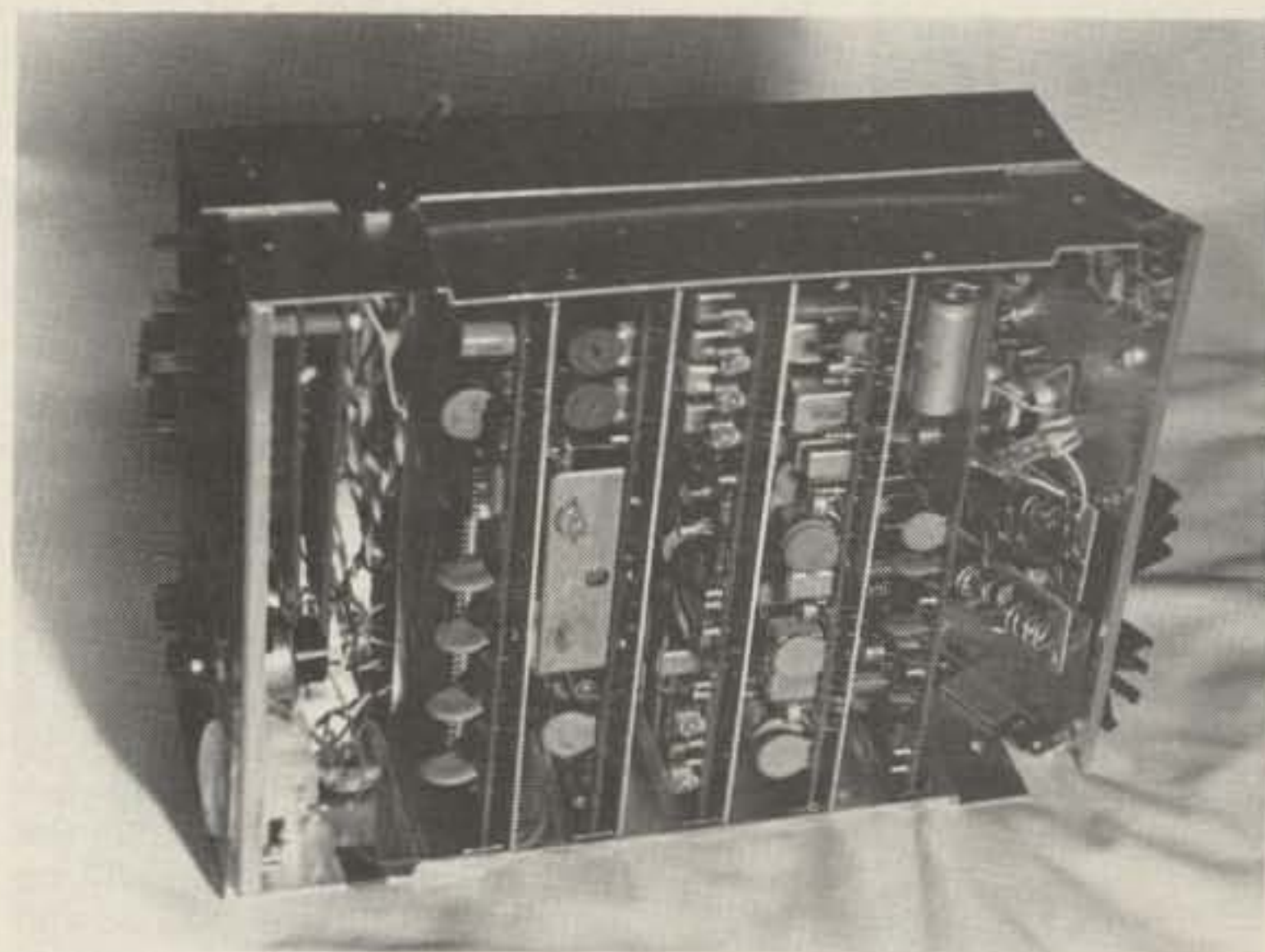
Photo C. Top cover removed to show swing-out panels and T-R relay.
