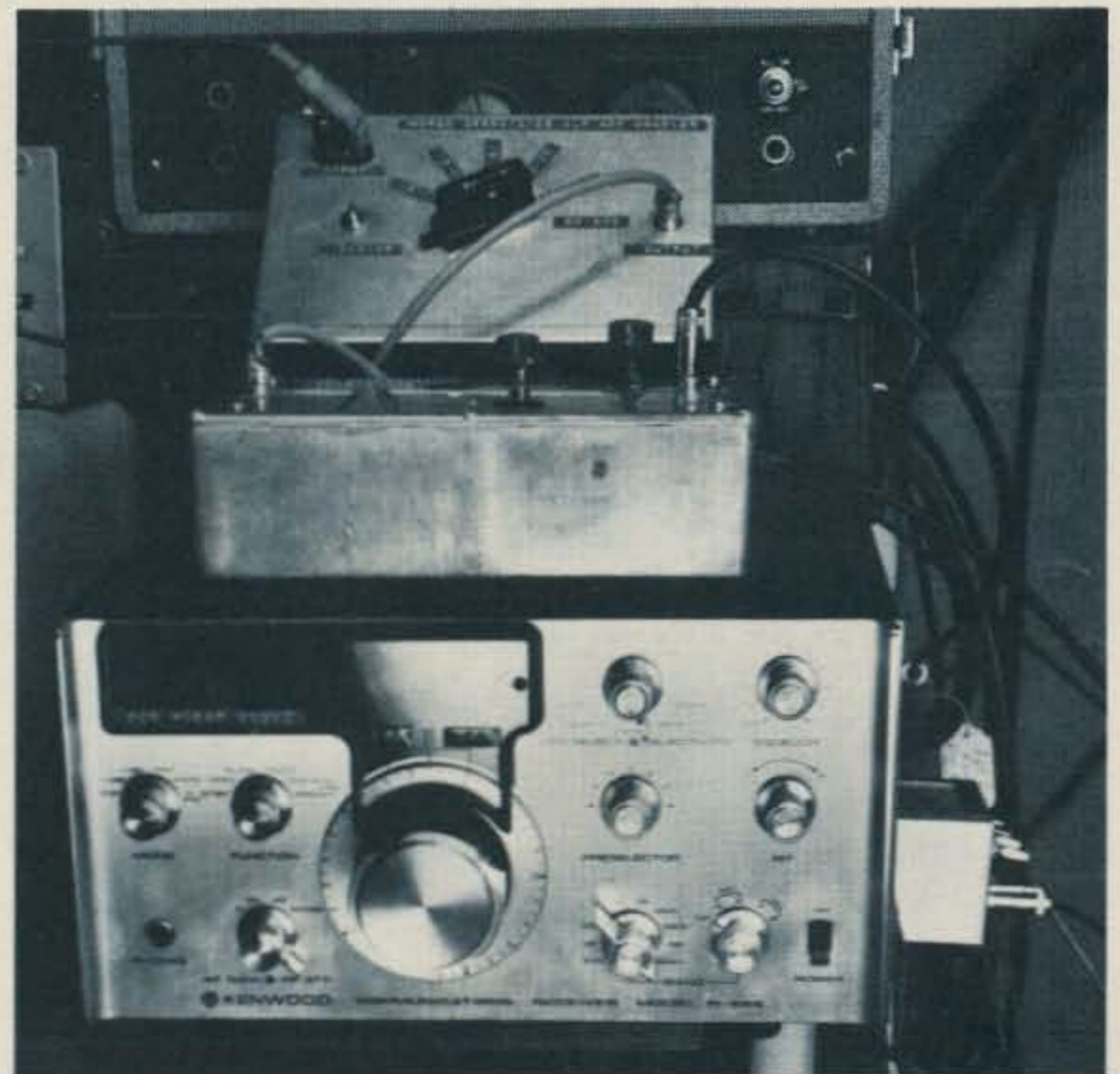
Photo C. The converter set up with the Kenwood R599 receiver. The antenna coupler can be seen at the top above the converter.
