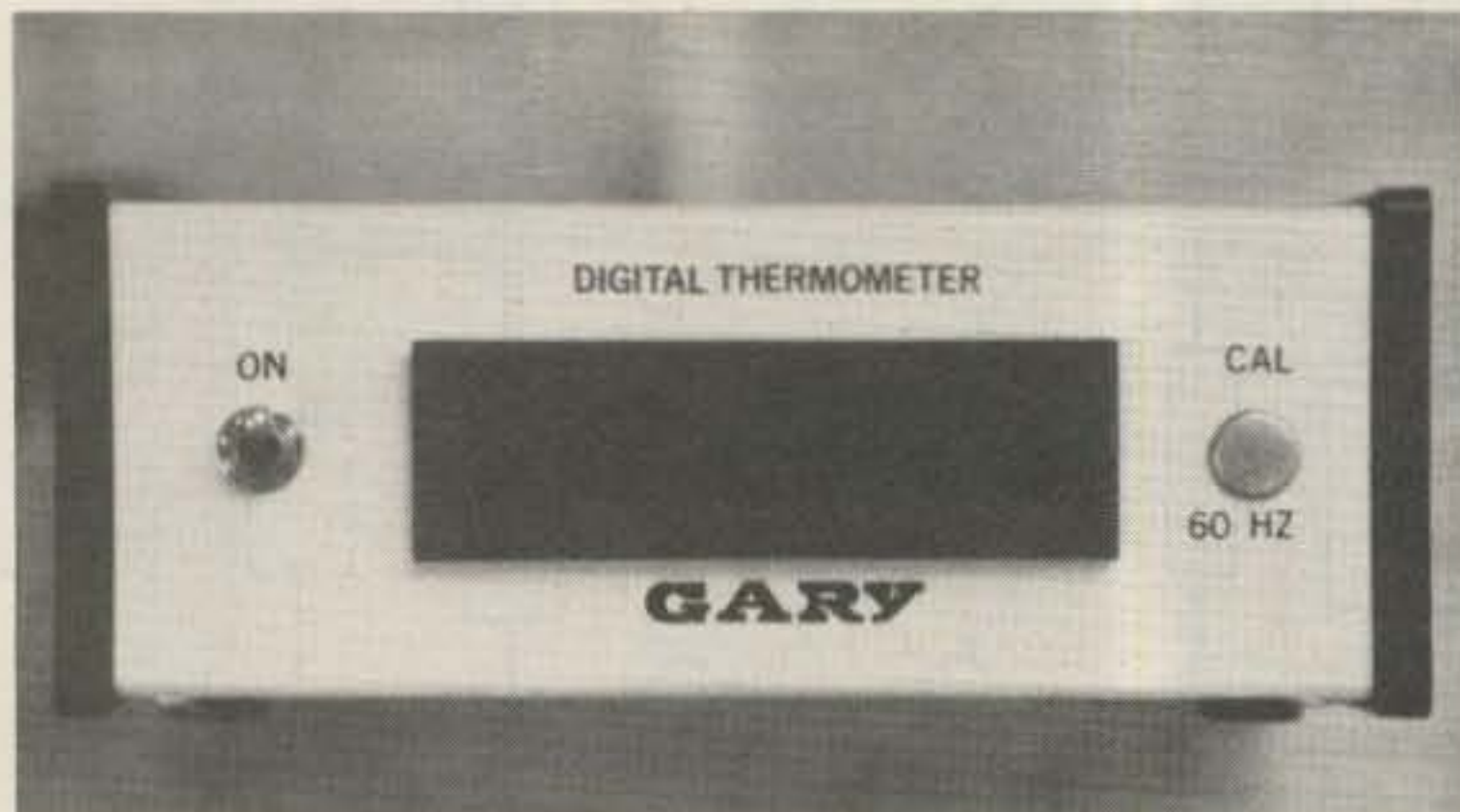
Here's an assembled digital thermometer. It gives good accuracy at a very low cost.
