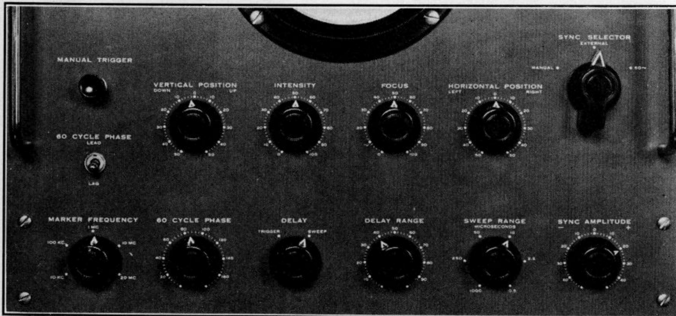
Figure 1. A portion of the control panel of the Type 293 showing, at extreme top-left, the manual trigger push-button.
