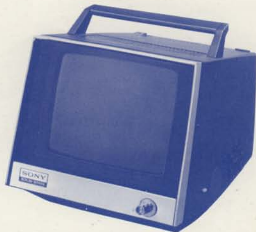
Compact and lightweight 7-inch monitor with high resolution, video only
