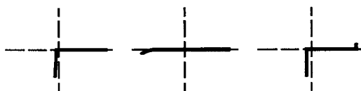
Type: Normal Diode High Voltage Diode Z-Diode 12V Terminals: Cathode-Anode Cathode-Anode Cathode-Anode Connections: (CT-GD) (CT-GD) (CT-GD)
