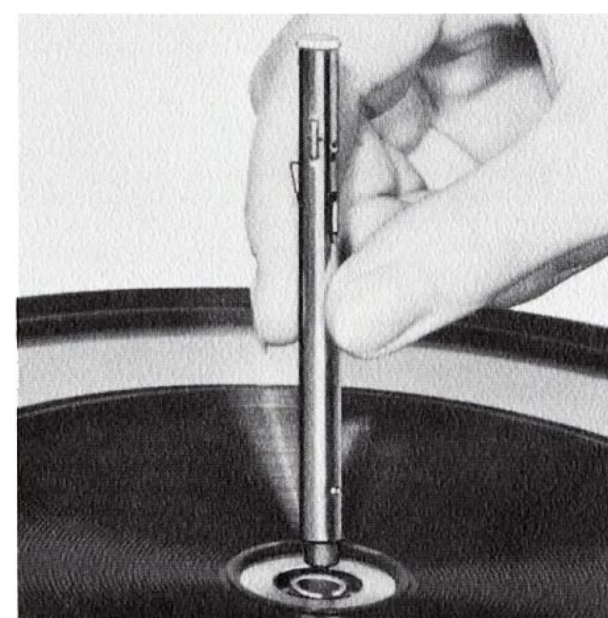
Fig. 29. Multiple-play spindle holds up to six records.
