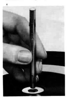
Insert the changer spindle by placing the key at its base into the slot of the shaft. Then turn the spindle clockwise until it stops. Up to six records can be placed on the spindle.
