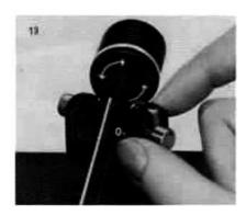
With the tonearm balanced at zero, you now set both tracking force and anti-skating simultaneously by turning the calibrated dial to the number you want. This is accurate to within 0.1 gram. (Follow the instructions with your cartridge for the recommended tracking force.)
