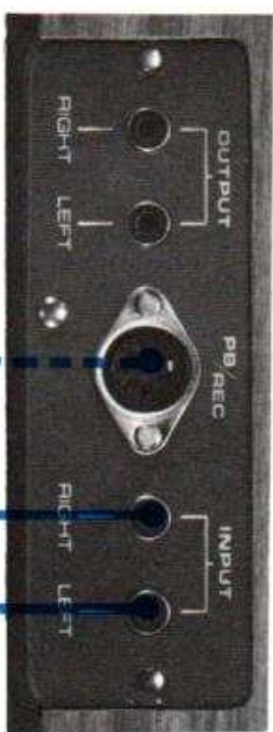
Connect desired source with RCA/RCA connection cord.
