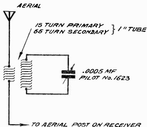
*This simple wave trap will help eliminate interference from strong local stations.*
