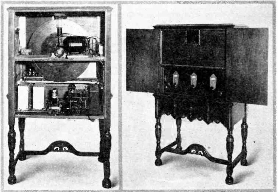
*This television receiver made history in 1928 when it was used at New York University in the Fall of 1928 for the first public demonstration of radio television staged in the East. It successfully reproduced 1½-inch images broadcast from station WRNY by the transmitter pictured on page 30. The instrument was constructed in the Pilot laboratories.*
