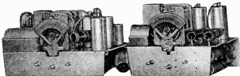
*The chassis of the "All-Wave" out of the cabinet. Left, the 7-tube broadcast unit; right, the four-tube short-wave converter. Four of the coils of the latter unit are visible at the extreme right.*
