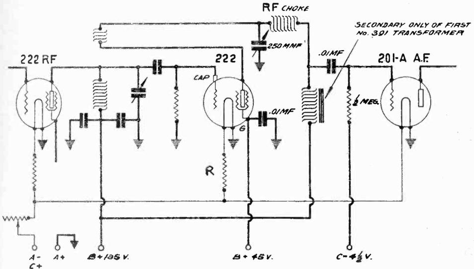
This diagram shows how a screen-grid detector is used in the K-110 model Super-Wasp. The rest of the R.F. and A.F. connections remain the same as before.
