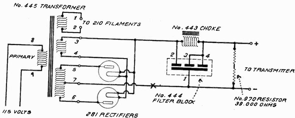
Schematic diagram of the heavy duty power pack. A single pole switch should be connected at the point marked X in the negative lead.
