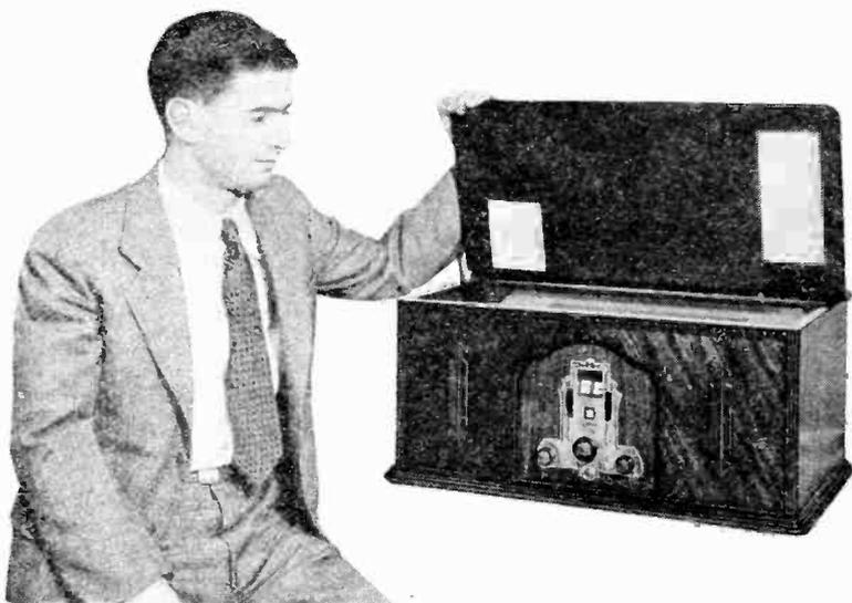
*His Majesty's personal short-wave receiver, a Pilot "All-Wave". The white areas on the cover are pieces of asbestos that protect the wood from the heat of the 280 and 245 tubes.*
