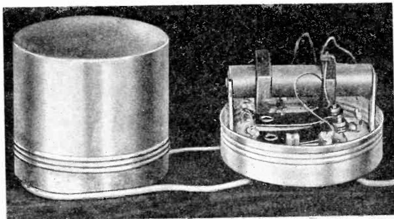
*A close-up of one of the intermediate frequency transformers used in all the Pilot super-heterodyne receivers. The two coils are wound on an impregnated wooden form. The small balancing condensers are just underneath.*
