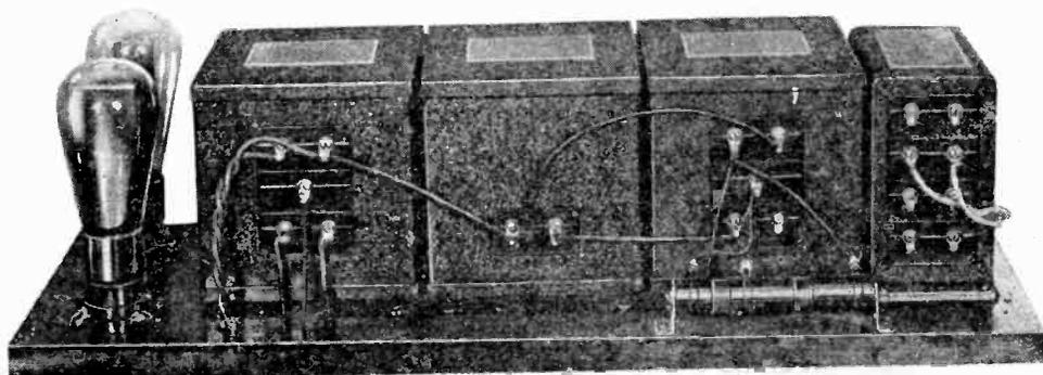
*The simple "breadboard" layout of the power pack makes wiring easy. Left to right: 281 rectifiers, No. 441 power transformer (replaced by the No. 445 since this picture was taken), No. 443 choke, No. 444 filter block; No. 446 transformer (now unnecessary). The No. 970 resistor is in front of the filter block.*
