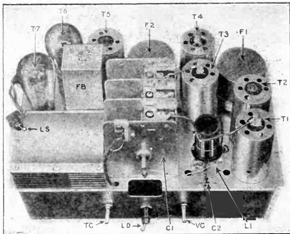
A close-up of the seven-tube super-heterodyne chassis, with all the parts marked to correspond with the designation on the schematic diagram on the next page.
