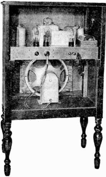
*Back view of the Pilot 10-tube Console, showing the arrangement of the chassis and the nine-inch dynamic speaker.*
