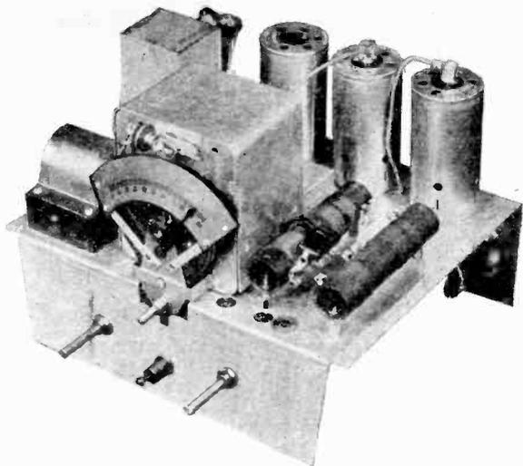
*Left: A close-up of the short-wave converter chassis. The four tubes are along the back edge, the coils above and below the chassis in the right foreground. Below: the under side of the chassis, showing the other three coils grouped around the wave-changing switch.*
