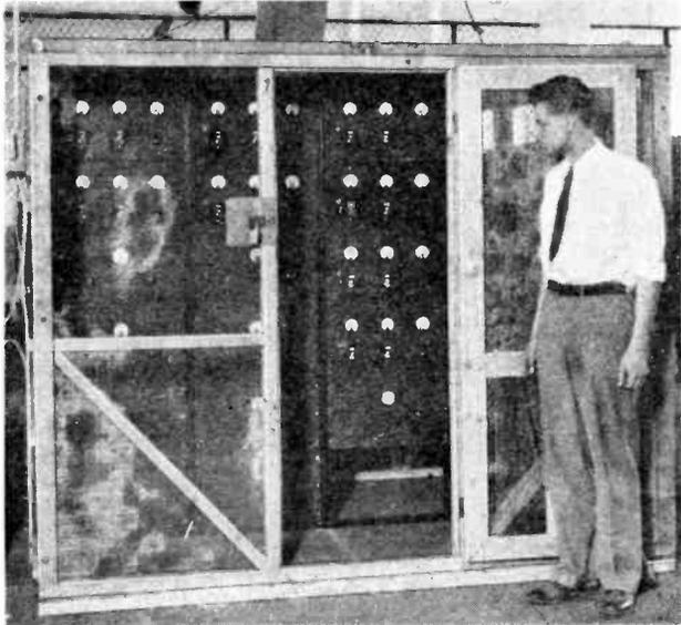
*Left, Fig. 5: The signal generating booth, containing half a dozen miniature transmitters, all crystal-controlled. These are connected by shielded cables to the test cages pictured in Fig. 6. This complicated apparatus was designed and constructed by J. L. Montgomery, who is shown in the photograph.*
