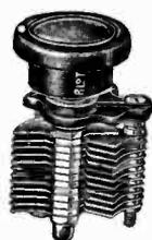
There are four sizes: the J-5, having a maximum capacity of 15 mmf.; the J-7, 25 mmf.; the J-13, 50 mmf.; and the J-23, 100 mmf. The catalog numbers indicate the number of plates. The instruments themselves are approximately 1½ inches on end and 1 to 1¾ inches deep, depending on capacity.
