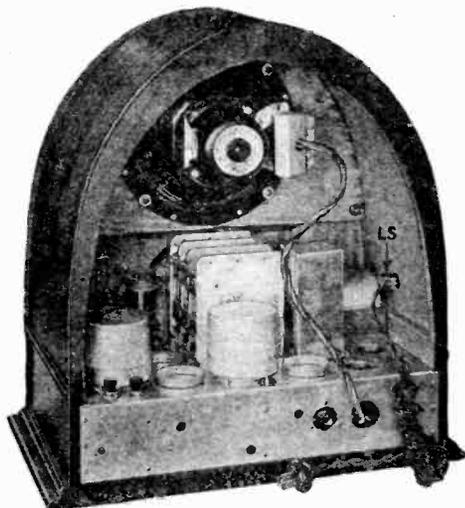
Back view of the Pilot Midget super-heterodyne, showing the arrangement of the chassis and the loud speaker. LS is the line switch.
