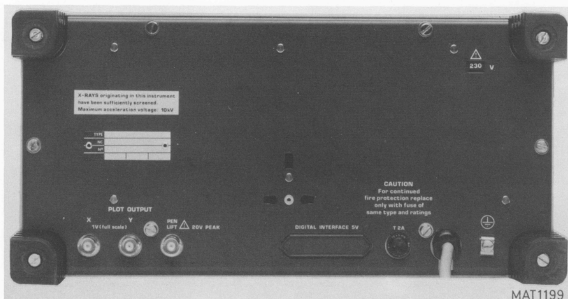
Fig. 2.1. Rear view of oscilloscope showing mains adaptor switch and fuse.
