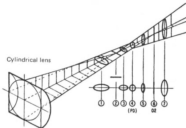
Fig.3-33 Cylindrical lens
