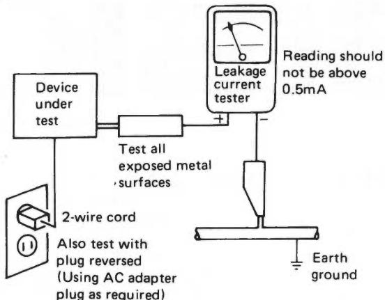
ANY MEASUREMENTS NOT WITHIN THE LIMITS OUTLINED ABOVE ARE INDICATIVE OF A POTENTIAL SHOCK HAZARD AND MUST BE CORRECTED BEFORE RETURNING THE APPLIANCE TO THE CUSTOMER.
