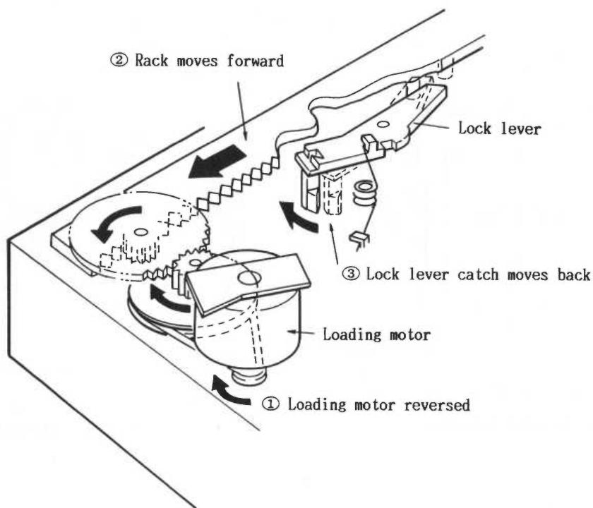
Fig.3-14 Eject operation (1)
