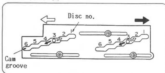
When the stairs (left and right sides) move back and forward, the 6-step cam grooves force chassis projections up and down to raise and lower the servo mechanism.
