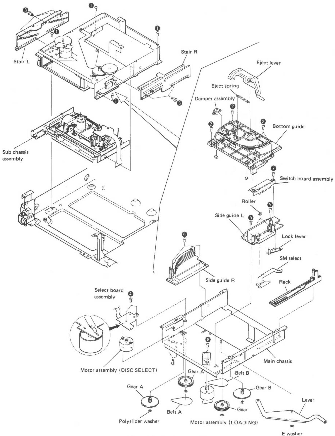
Fig. 4-2 Mechanism assembly
