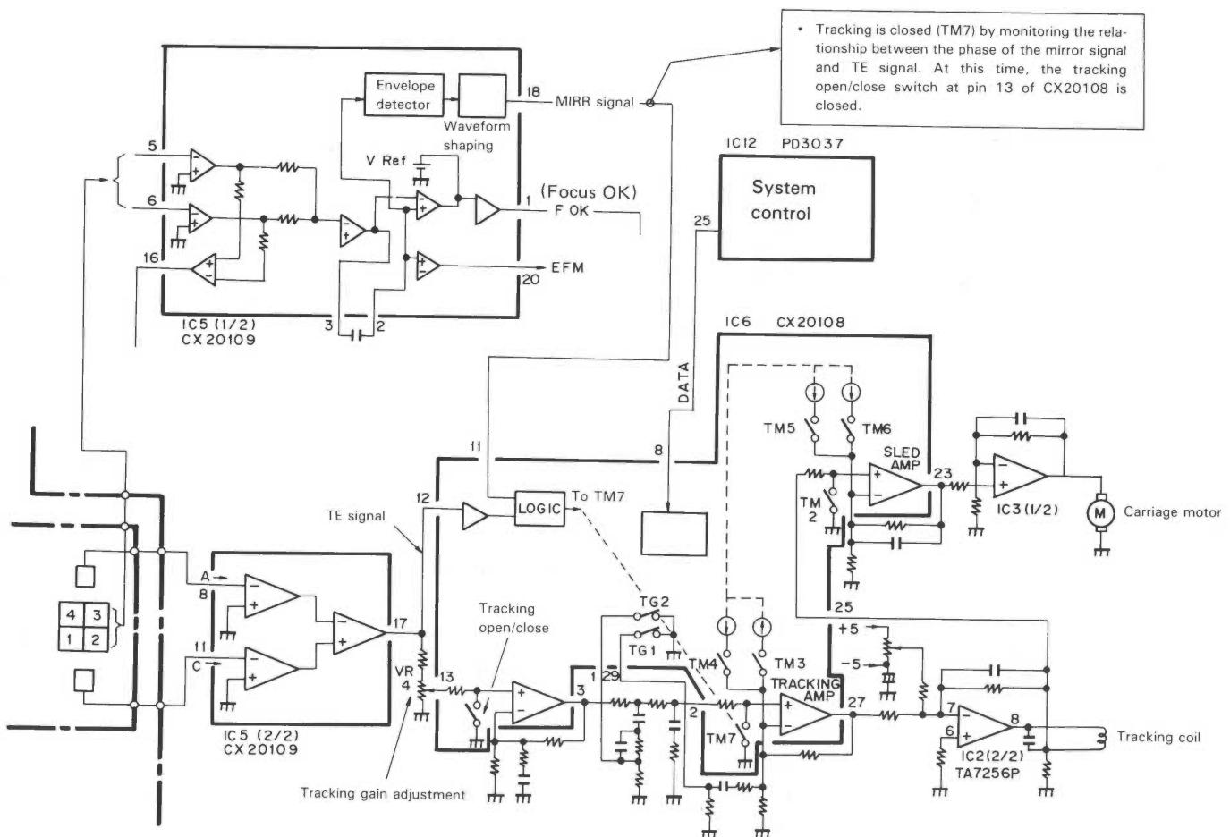
Block diagram of tracking servo
