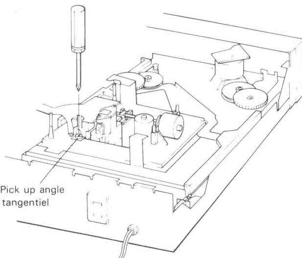
Fig. 10-5 Réglage pick up angle
