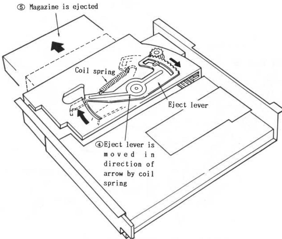
Fig.3-15 Eject operation (2)
