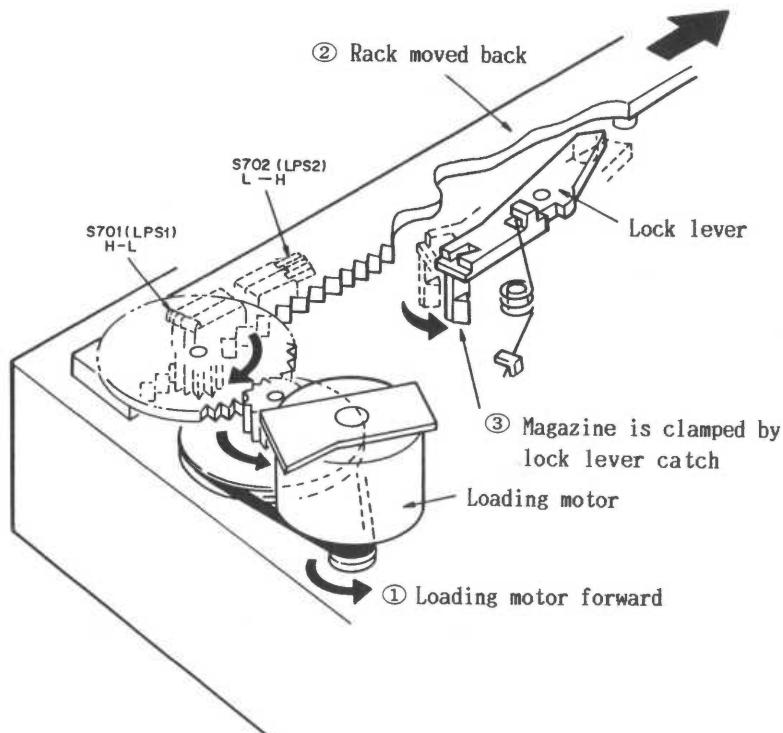
Fig.3-8 Loading operation
