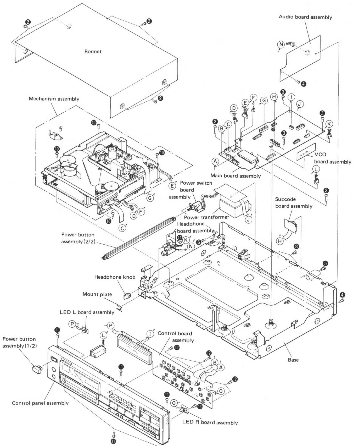
Fig. 4-1 Disassembly
