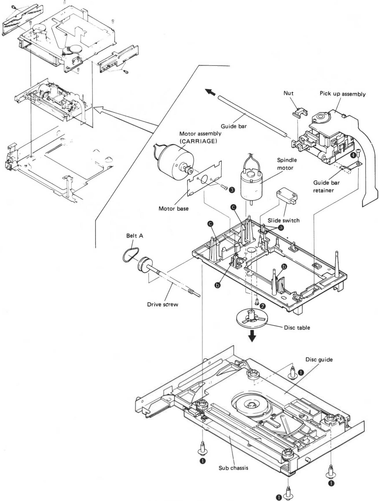
Fig. 4-3 Disc table assembly
