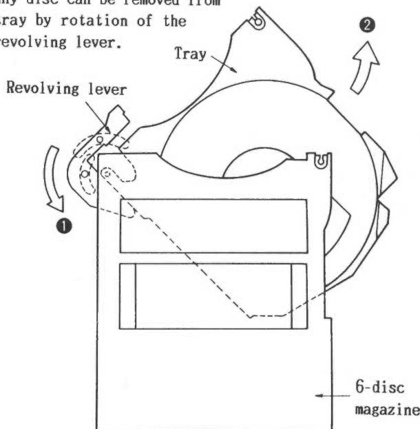
Fig.3-11 Revolving lever movement
