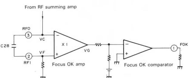
Fig. 3-13 Focus OK circuit
