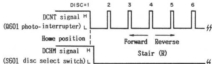
Fig.4-1 Stair (R) movement timing
