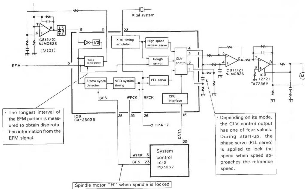
Block diagram of spindle servo
