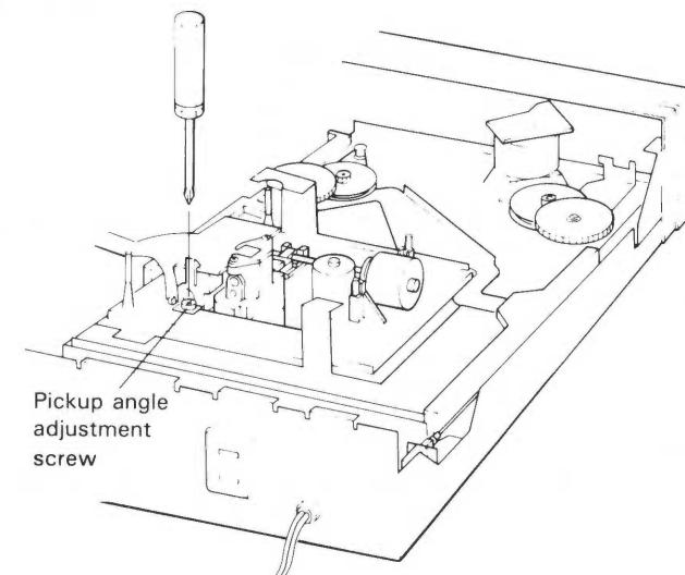
Fig. 10-5 Pickup Angle Adjustment
