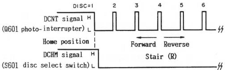
Fig.3-6 Disc count pulse
