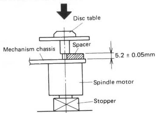
Fig. 4-3 Disc table assembly
