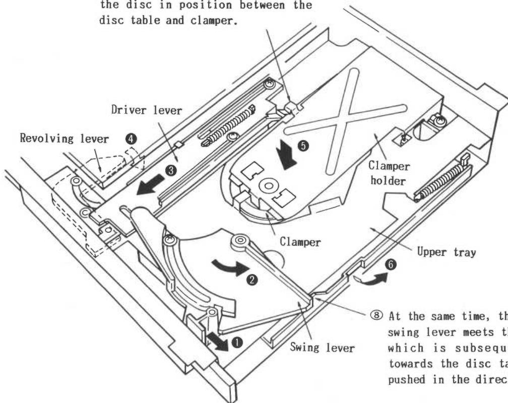
⑧ At the same time, the edge of the swing lever meets the upper tray which is subsequently moved towards the disc table by being pushed in the direction of arrow 6
