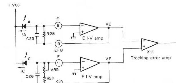
Fig. 3-12 Tracking error amp circuit
