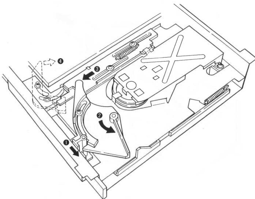
Fig.3-10 Swing lever movement (2)
