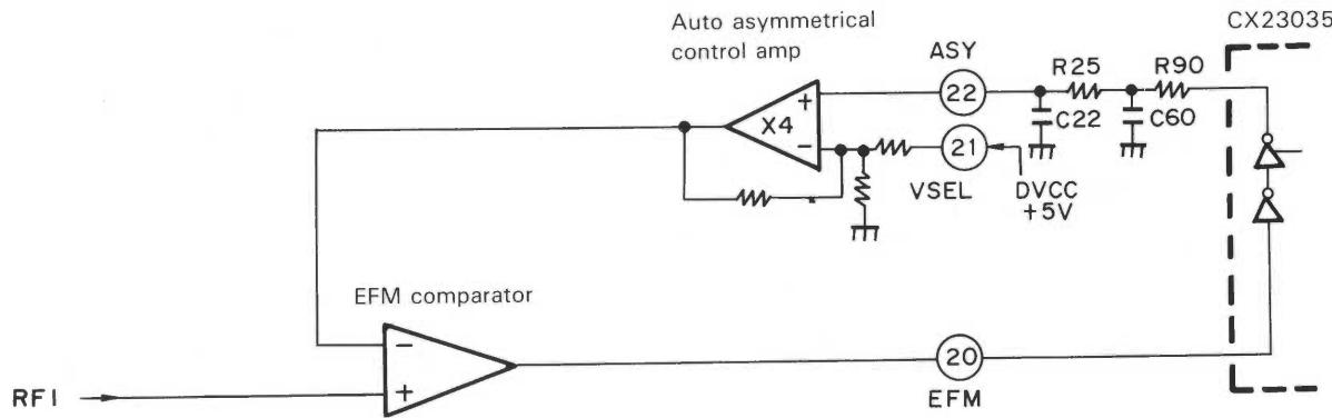
Fig. 3-15 EFM comparator circuit
