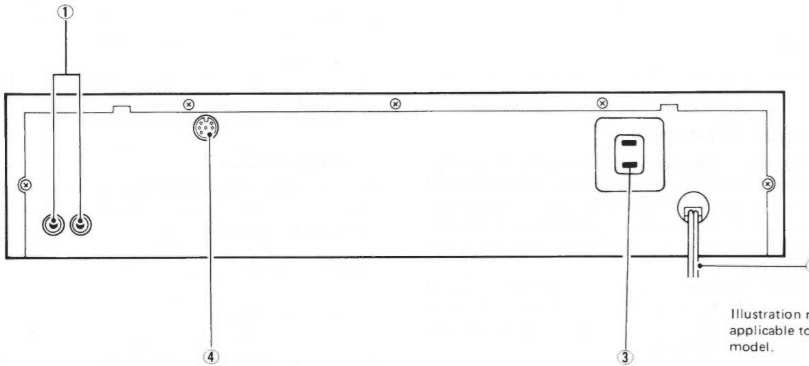
**① AUDIO OUT terminals****② Power cord****③ AC OUTLET (UNSWITCHED, MAX. 100 W)**
