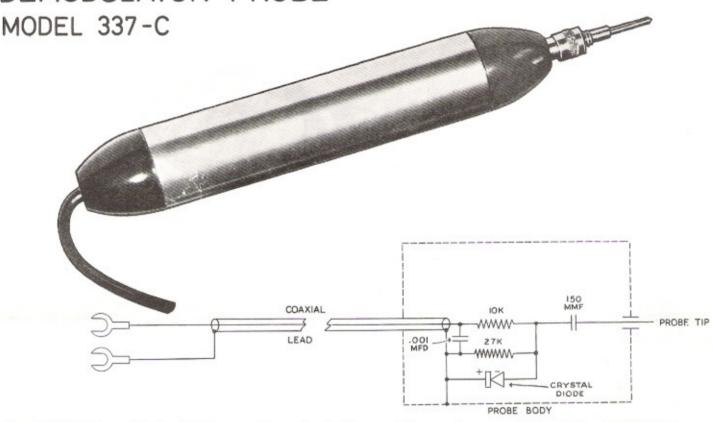
The #337-C Demodulator Probe greatly extends the usefulness of any oscilloscope. It provides a means of showing modulation envelopes of RF or IF carriers as found in radio and television receivers. Thus the oscilloscope can be used as a signal tracer, a gain analyzer and an alignment indicator. Many other uses will become evident as the user becomes more familiar with the characteristics of the probe and oscilloscope combination.
