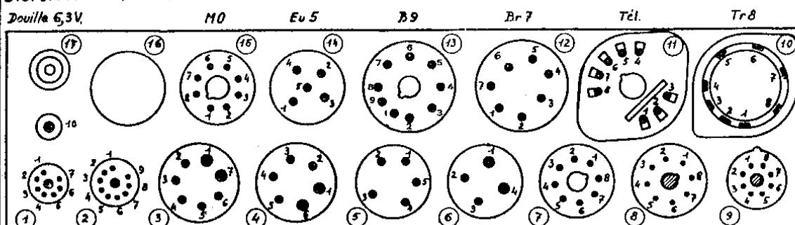
**NUMEROS DES ELECTRODES DES SUPPORTS - CORRESPONDANCE AVEC LES LAMPES VUES PAR DESSOUS**
