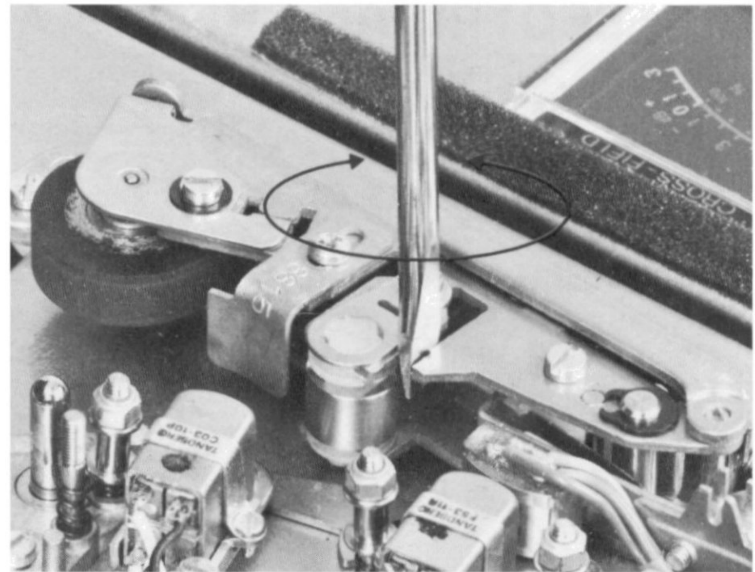
Fig. 2.16. Azimuth adjustment of inertia idling roller.
