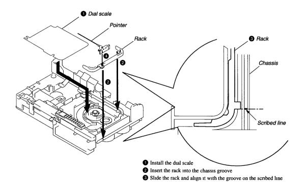
4 Line up the groove on the pointer with the matching portion on the rack and fit it in
