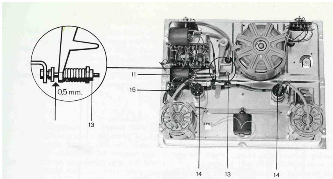
The end-of-tape switch and its operating lever are then properly adjusted when the switch remains open (or closed on older models) for any movement of the sensing lever inside the tape-guide post. Accidental tripping due to sticky splices etc. will thus be avoided.
