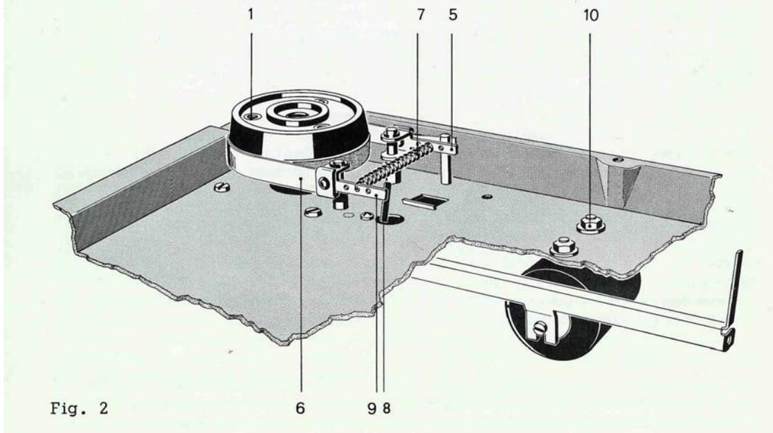
It is important to check that the brake band (6) is running flat on the brake lining and not biting on the upper or lower edge. Adjust alignment of brake band by slightly pivoting it in the rivets if required.
