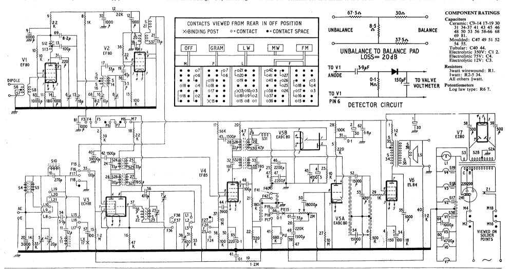
unmodulated to g1 V3 via a 1,500pF ceramic capacitor. During alignment, input should be such that the voltage across C4 does not exceed 8V.
