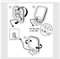
Position the antenna as far as possible from a TV, VCR or other radiation source.
