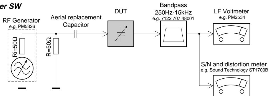
To avoid atmospheric interference all AM-measurements have to be carried out in a Faraday's cage.
