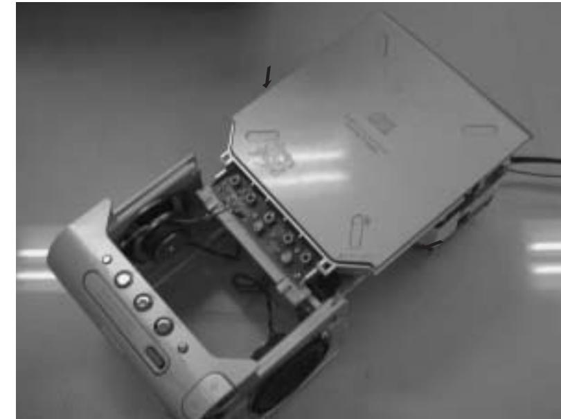
**C. REMOVE DECK MECHANISM**
