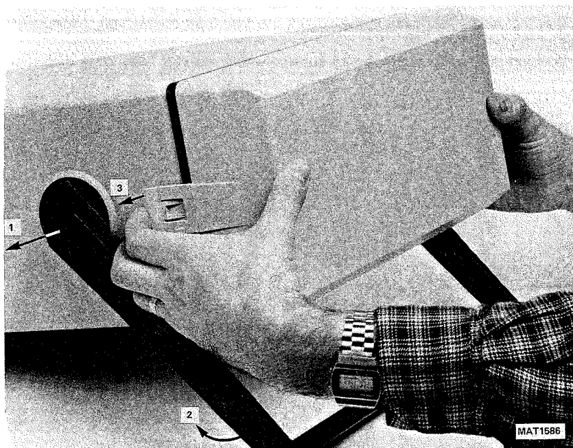
Fig. 3.2. Removing the front cover
