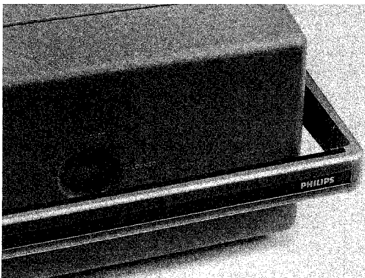
Fig. 2.1. Removing the front cover.
