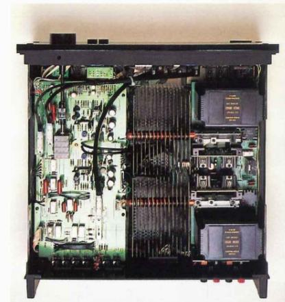
Interior of L-01A pre-main amplifier eliminates distortion with separate power sources via non-magnetic body.
