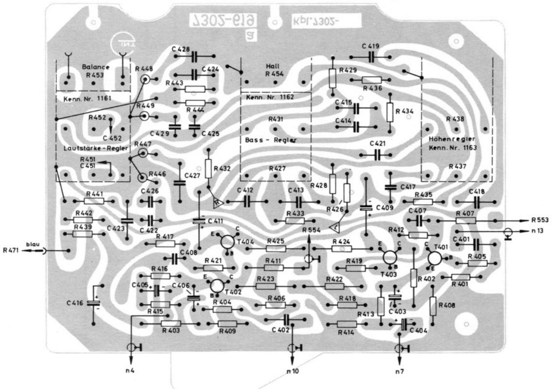
CIRCUIT IMPRIME PRISES DE RACCORDEMENT, VU DU COTE SOUDURES
