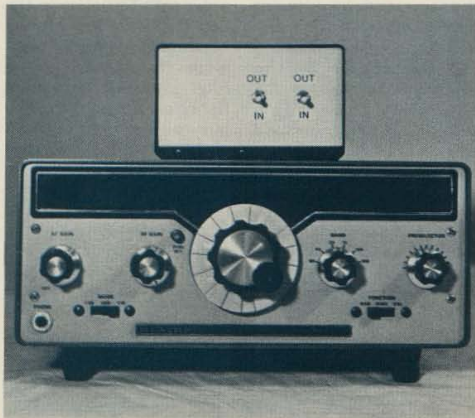
Photo B. Front view of modified HR-1680 (with completed filter-blanker on top) shows details of modified spinner knob.
