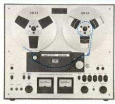
Place a full reel of tape on the Supply Reel Table and an empty reel on the Take-Up Reel Table. Thread the tape as illustrated by the dotted lines in the figure. Lock reels into place with Reel Retainers provided on reel shafts.
