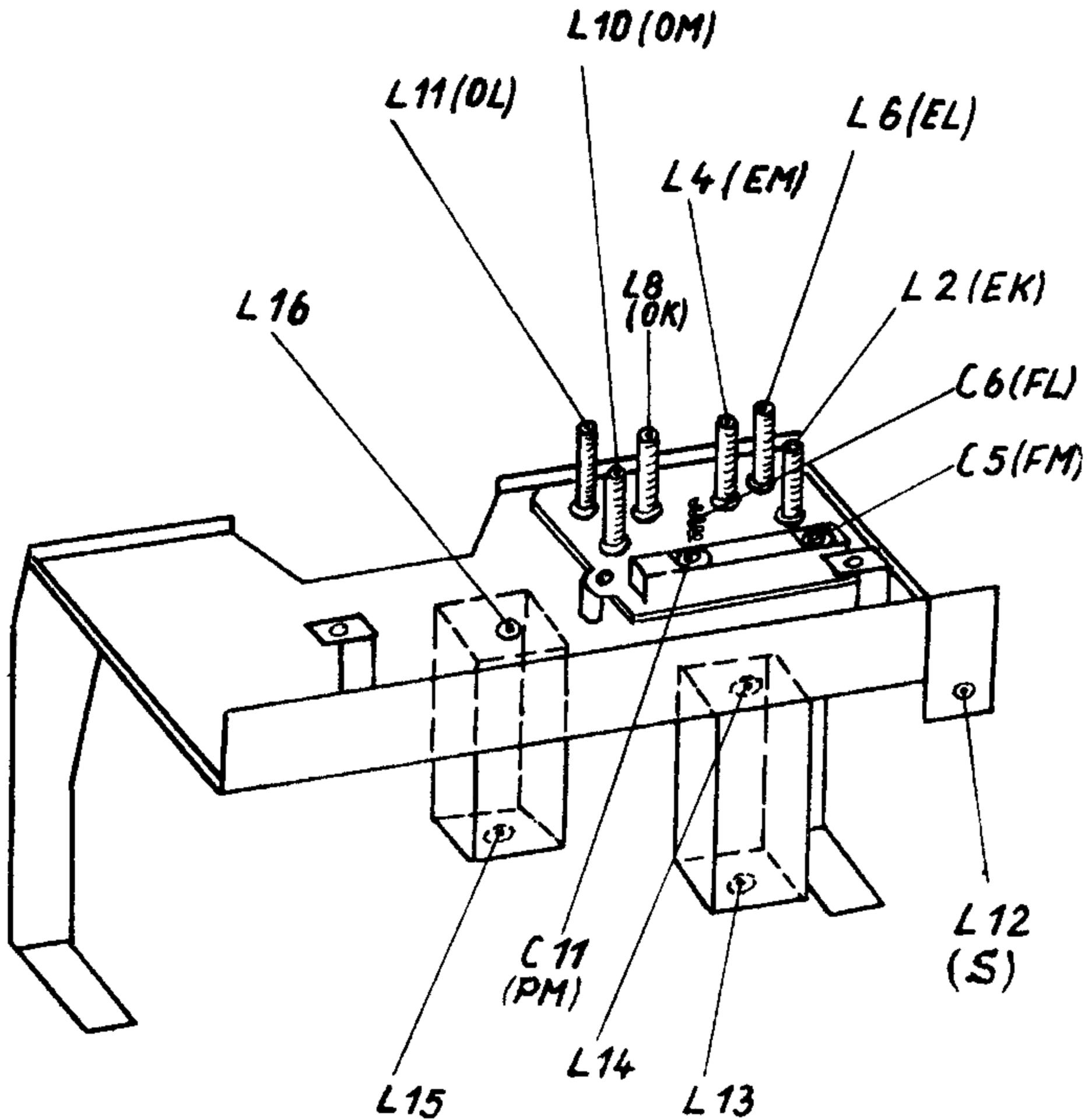
Zwischenfrequenz: 468 kHz L 16, L 15, L 14, L 13
