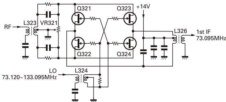
Fig. 7 First mixer circuit of the RX-2 path
