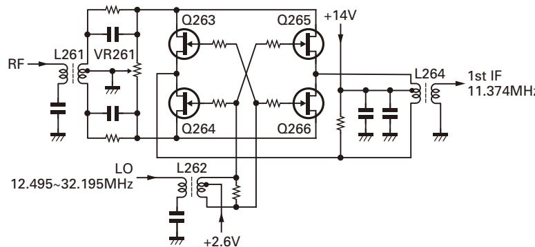
**Fig. 6 First mixer circuit of the RX-1 path**
