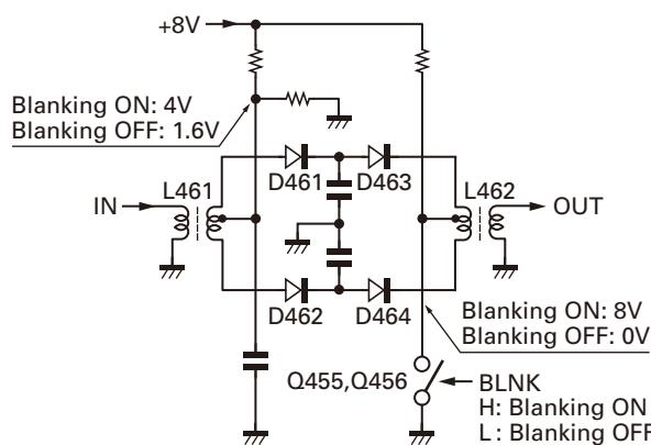
Fig. 11 Blanking circuit
