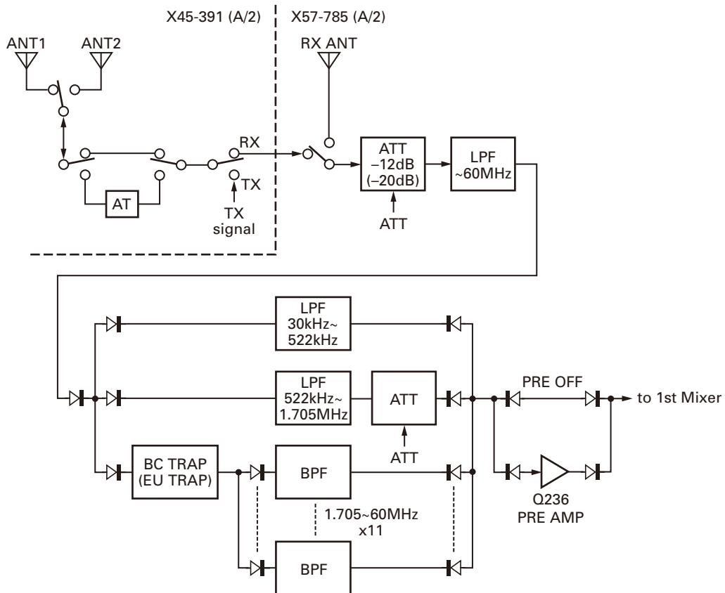
Fig. 3 From antenna terminal to preamplifier (Q236)
