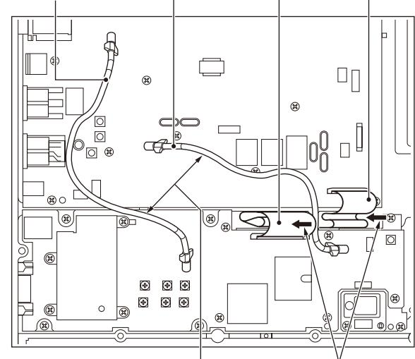
Separate the two coaxial cables
