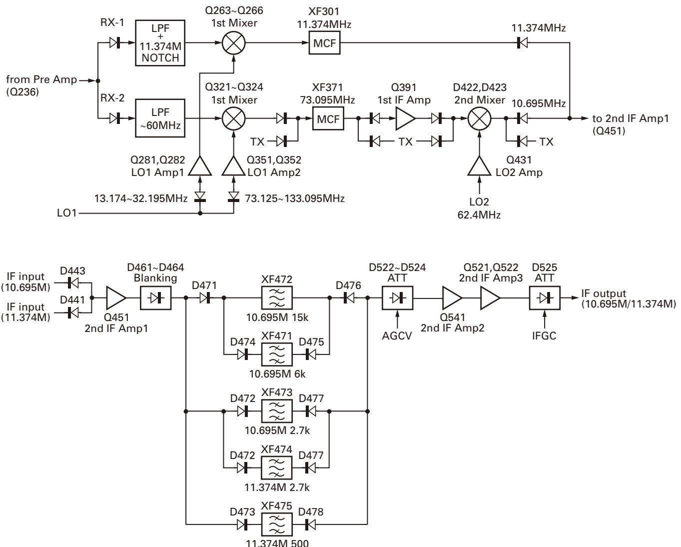
Fig. 4 From the preamplifier (Q236) to the second IF frequency (10.695MHz/11.374MHz)
