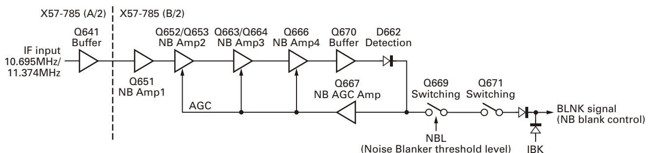
Fig. 10 Noise detection circuit
