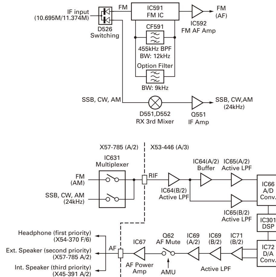
**Fig. 5 From second IF to AF output**
