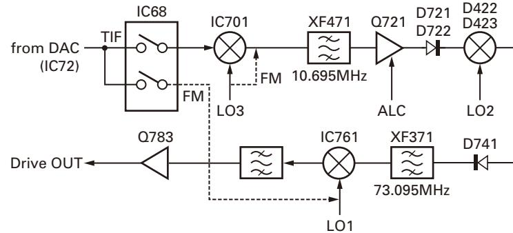
**Fig. 12 From transmission signal (TIF) to drive output**
