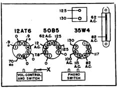
Voltage measured from socket terminal to point marked "X". Large numerals indicate readings with vacuum tube voltmeter. Small numerals indicate readings with 1000 ohm-per-volt meter.
