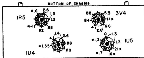
\* If taken with a 1000 ohm-per-volt meter, readings will be lower or zero.
