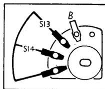
Diagram of the tone control switch unit, drawn as seen from the rear of the chassis deck.
