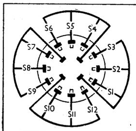
Diagram of the waveband switch unit, as seen from the rear of an inverted chassis. The associated table is on the right.
