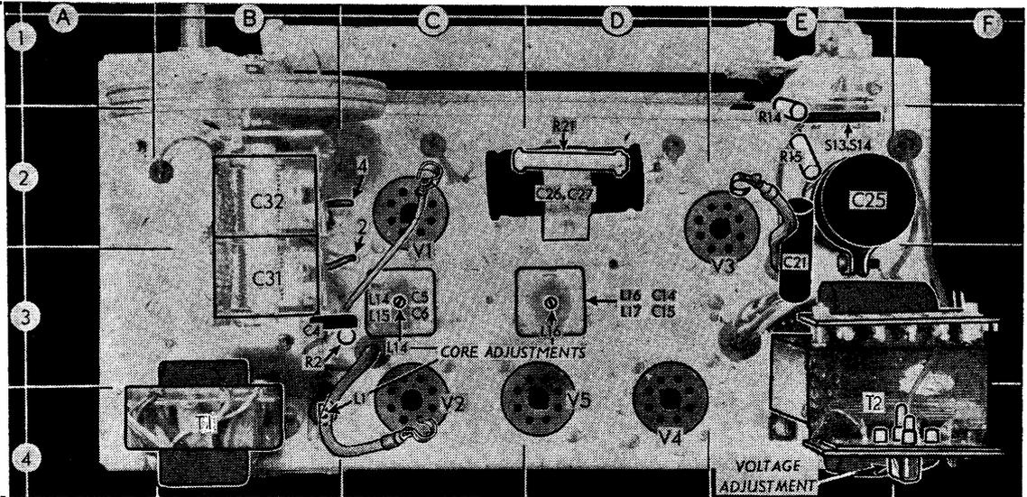
ling capacitor C19 and C.G. resistor R9 to control grid of triode section, which operates as A.F. amplifier. I.F. filtering by C16, R6 and C17 in diode circuit. Provision for the connection of a gramophone pick-up across R8.
