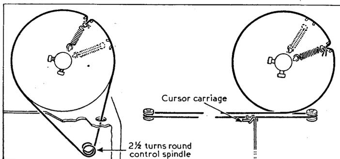
Sketches showing the main gang (left) and scale cursor (right) drive cord systems as seen from the front when the gang is at maximum. Each has its own tension spring.
