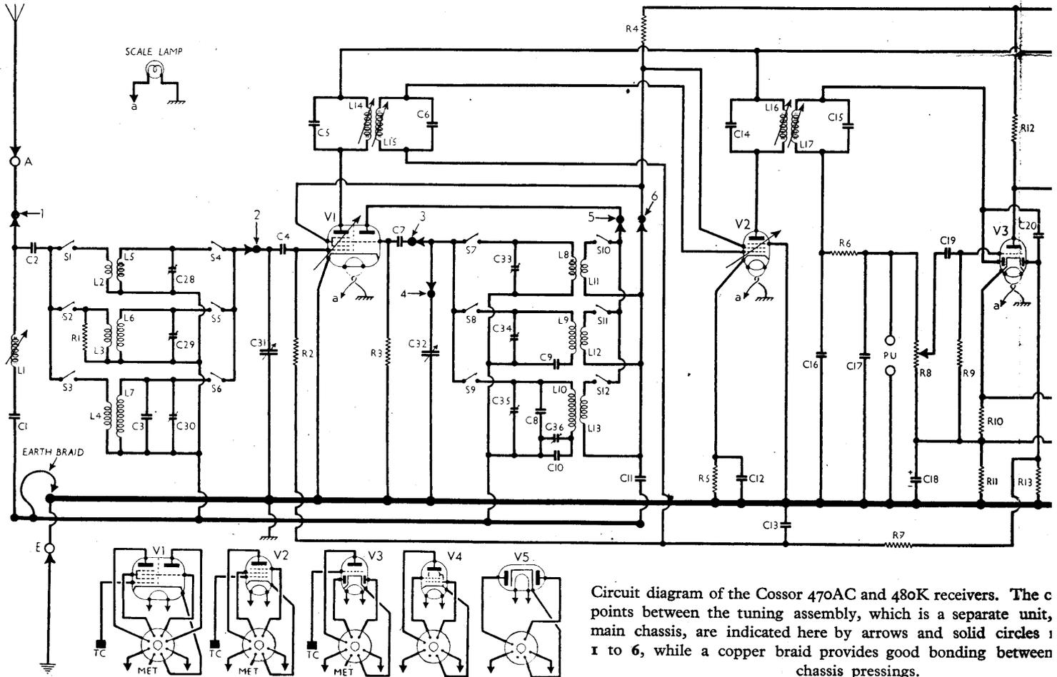
Circuit diagram of the Cosmor 470AC and 480K receivers. The c points between the tuning assembly, which is a separate unit, main chassis, are indicated here by arrows and solid circles 1 to 6, while a copper braid provides good bonding between chassis pressings.
