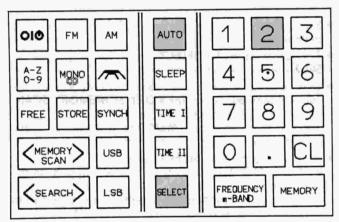
Please observe that the SELECT button must be pressed after termination of the check to switch back to normal operation.
