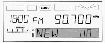
During this function, the station tuned to last remains always temporarily stored on button "0" of the numeric buttons ("Manual Tuning Memory" HA) in the waveband concerned.
