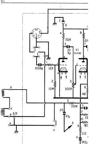
Record/playback tape test. Feed in signal of approximately 50mV at 1kc/s to microphone socket, 100K in series, and adjust recording level. Reduce input by 20dB (10:1) and record following frequencies: 60c/s, 125c/s, 333c/s, 1kc/s, 2kc/s, 4kc/s, 6kc/s, 8kc/s, 10kc/s, 12kc/s. Playback output must be within +3dB -5dB.
