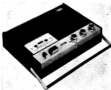
Philips version of twin-track cassette recorders which are styled in black polystyrene cabinets with brushed aluminium trim. ST9112AT includes mains supply unit and pilot lamp
