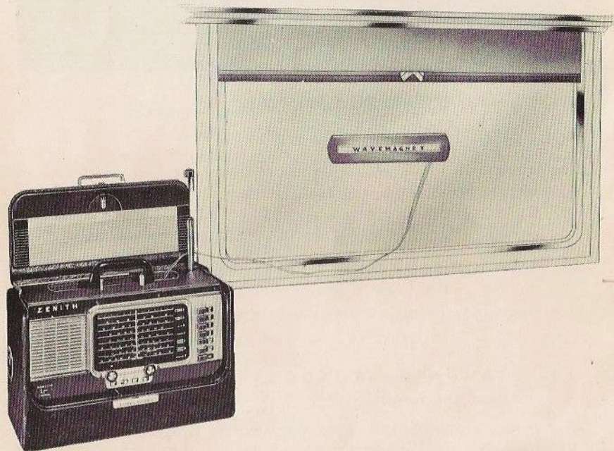
Figure 16—Detachable Wavemagnet in Position on a Window.
