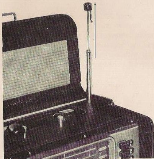
Figure 18—Waverod Must Be Extended for Shortwave Reception.
