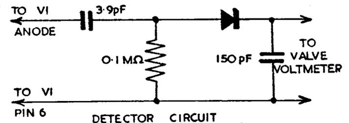
Check that the response is straight over approximately 200 kc/s. Apply A.M. (modulation 400 c/s depth 30%). The straight part of the curve should remain unchanged.
