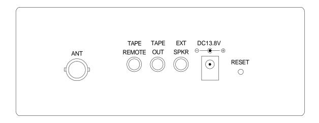
ANT -- connect optional antenna with BNC connector.
