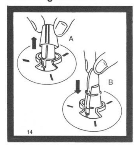
The platter is secured to the chassis by a spring-clip around the groove of the shaft. To remove the platter, use the special accessory cone supplied in the bag with the cartridge mounting hardware. Remove the spring clip as shown in Fig. 14 a. Then lift the platter slowly and gently off the shaft. Avoid touching the inner surfaces with your fingers, as skin oils can induce slippage.
