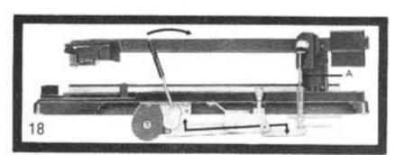
Cue-Control is shown at position , with tonearm supported by piston (A). When Cue-Control is shifted to position , the piston is released and permits tonearm to slowly lower to record. At this point, the tonearm is completely disengaged from the Cue-Control.
