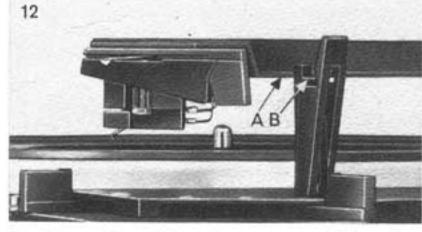
4. To raise the tonearm, slide the counterbalance back. To lower the tonearm, slide the counterbalance forward. (When points A and B as shown in fig. 12 are aligned, the tonearm is perfectly balanced.) Secure the balance by tightening the lock-knob.
