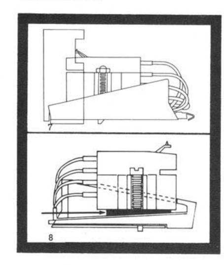
3. The specially tapered wedge, also supplied, is for use when you intend to play single records either exclusively or primarily. (Fig. 8) This wedge provides the optimum 15° vertical tracking angle when one record is on the platter. (However, even without the wedge, the vertical tracking angle will still be well within standard industry tolerances for single record play.)
