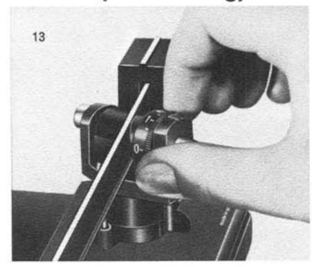
With the tonearm balanced at zero, you now set both tracking force and Tracking-Balance Control simultaneously by turning the calibrated dial to the number you want. This is accurate to within 0.1 gram. (Follow the instructions with your cartridge for the recommended tracking force.)
