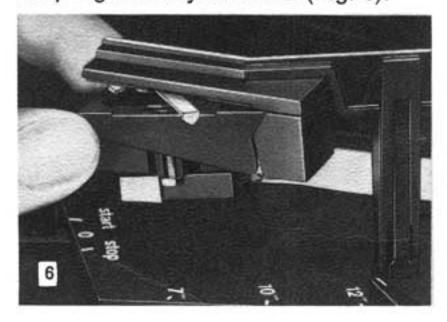
2. The special gauge supplied with your Dual, when snapped onto the holder as shown in fig. 7, will indicate the correct stylus depth for the cartridge when mounted. (Be sure the ridges on the inside of the gauge walls fit into the corresponding tracks on the side of the cartridge holder.)
