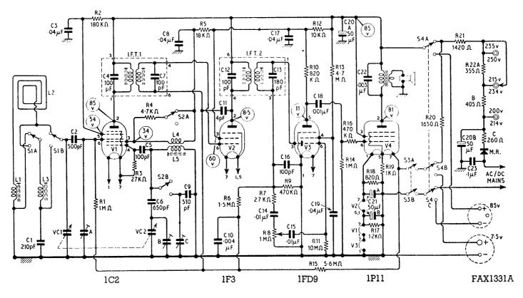
Figures in circles refer to the voltages on the various electrodes. All voltages were taken with an Avo 7 meter on the highest permissible range.
