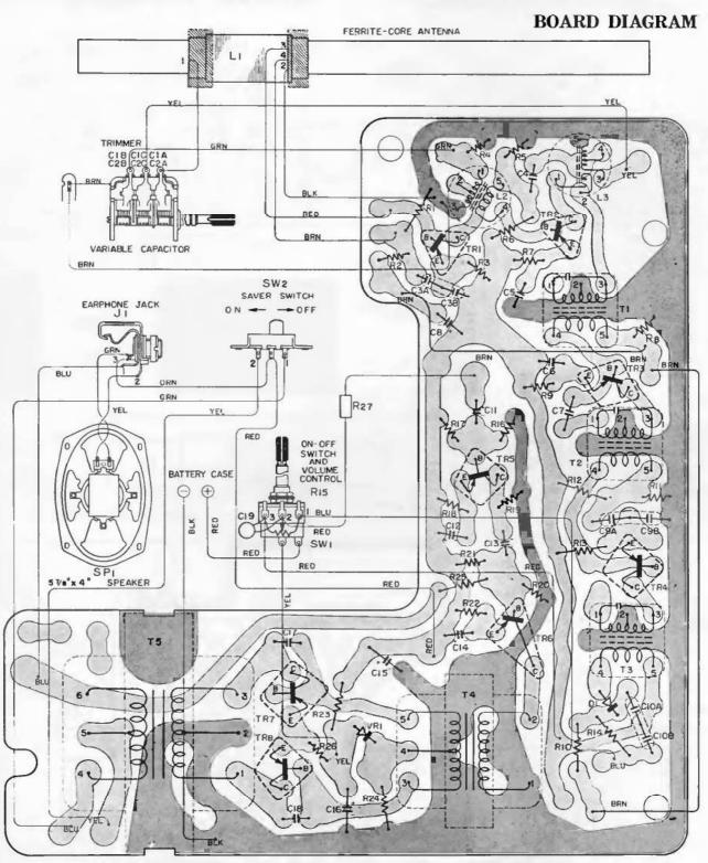
Signal tracing by injection of a signal from a signal generator is recommended as test procedure. The signal generator should be connected in series with a capacitor to avoid shorting out bias voltages. Of the transistors used in this receiver, the BASE is the signal input terminal (corresponding to signal grid of tubes), the COLLECTOR is the signal output terminal (corresponding to plate of tubes), and the EMITTER is the common terminal (corresponding to cathode of tubes),
