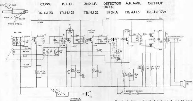
The output circuit used in this receiver is of the "Class B" type. It should be noted that in "Class B" output the battery current increases greatly with increased signal input.
