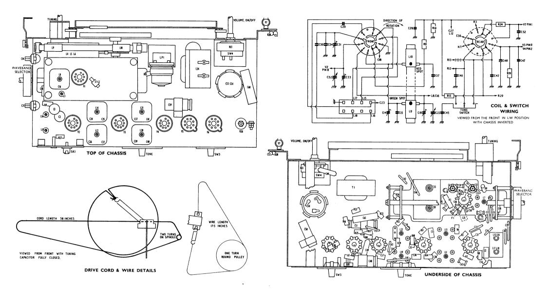
**A.M. A.G.C. AND TUNING INDICATOR:** From the diode load potentiometer, the rectified voltage is tapped off, filtered and applied as A G.C. voltage to the grids of V2 and V3. From the same tapping, a feed is taken, on positions 2 and 3 of SW2.C, to the grid of the tuning indicator.
