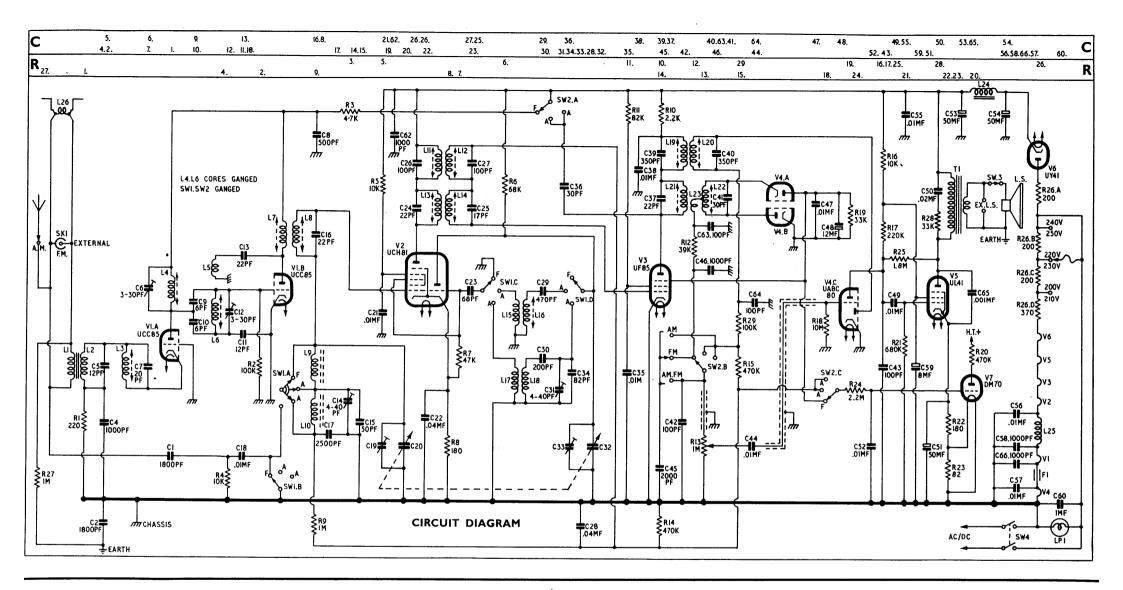
Correction: L18 should have iron dust core.
