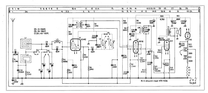
MODEL U195 is a four-valve, A.C./D.C. receiver offering switch-controlled selection of three M.W. and one L.W. stations. Built-in frame aerials are included for both M.W. and L.W. reception, and to cater for areas of low field strength, sockets are provided for the connection of an external aerial and earth.
